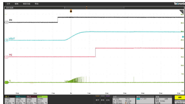
图 8-6. Start-Up Relative to EN Rising, I_{out} = 0\text{A} , PSM Mode
