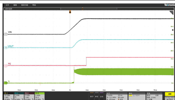
图 8-10. Start-Up Relative to Vin Rising, Iout = 7A
