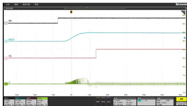
图 8-8. Start-Up Relative to EN Rising, Iout = 0A, OOA Mode
