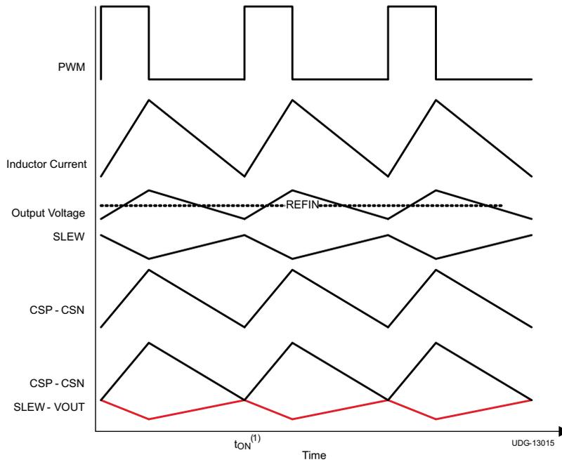
**Figure 30. On-Time Waveforms** <sup>(1)</sup>
