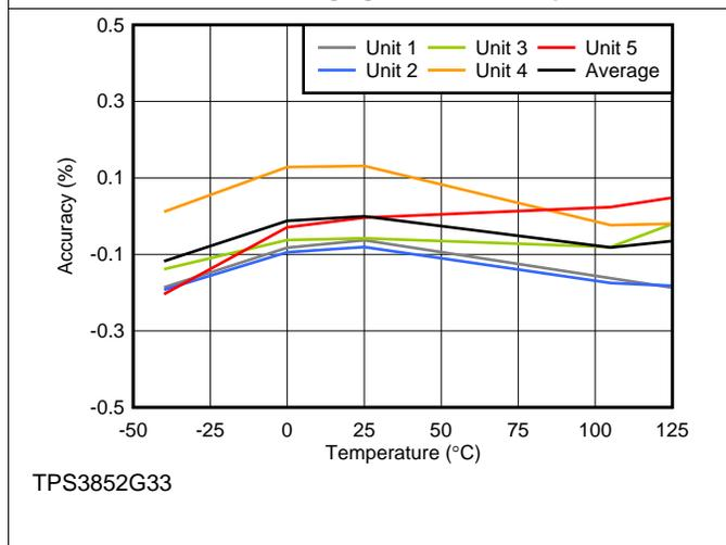
图 7. V<sub>ITN</sub> Accuracy vs Temperature
