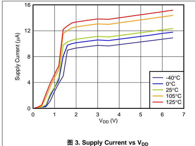
图 3. Supply Current vs V<sub>DD</sub>
