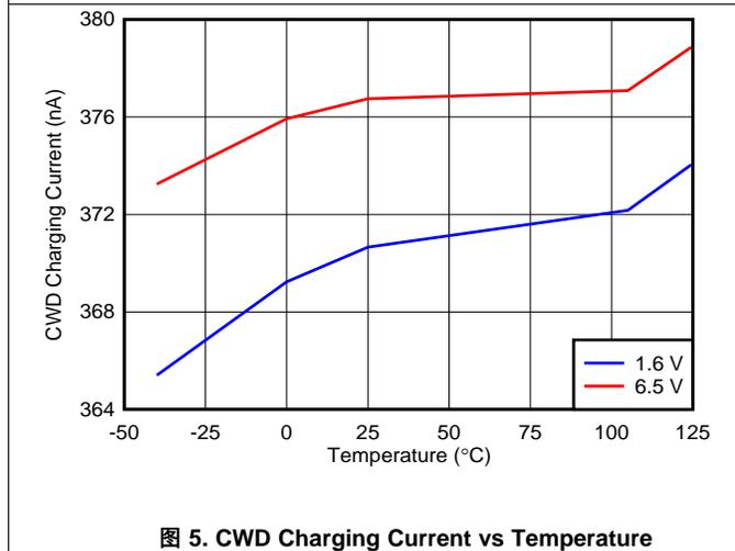
图 5. CWD Charging Current vs Temperature
