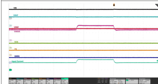
Device in steady-state, Load current ramped up from 50 A to 70 A for 10 ms and then ramped down to 50 A. OCP threshold set to 55 A, Overcurrent blanking delay set to 15 ms (OC_TIMER = 0x89)
