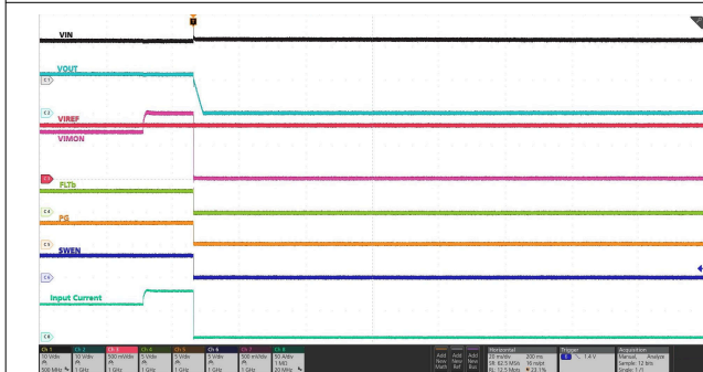
Device in steady-state, Load current ramped up from 50 A to 70 A for > 15 ms. OCP threshold set to 55 A, Overcurrent blanking delay set to 15 ms (OC_TIMER = 0x89), Latch-off configuration (Default, RETRY_CONFIG[5:3] = 000b)
