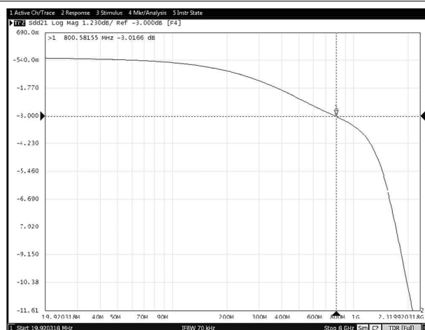
图 8-31. Data Transmission Characteristics vs Frequency (TPS25832-Q1)
