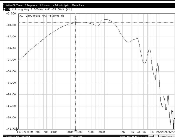
图 8-32. Off-State Data-Switch Isolation vs Frequency (TPS25832-Q1)
