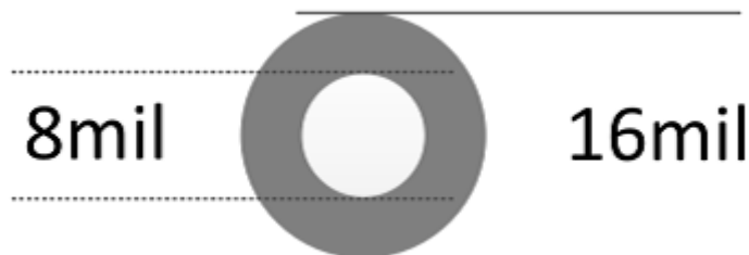
图 11-6. Recommended Minimum Via Sizing
