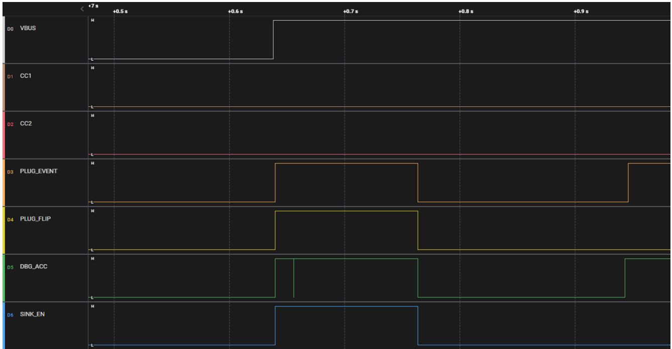
图 9-7. PLUG_EVENT, PLUG_FLIP, DBG_ACC, and \overline{\text{SINK\_EN}} - Debug Accessory Detection
