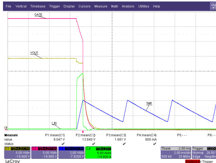
Figure 34. TPS2483 Retry-Cycle Timing Detail
