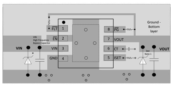
(1) Optional: Needed only to suppress the transients caused by inductive load switching.
