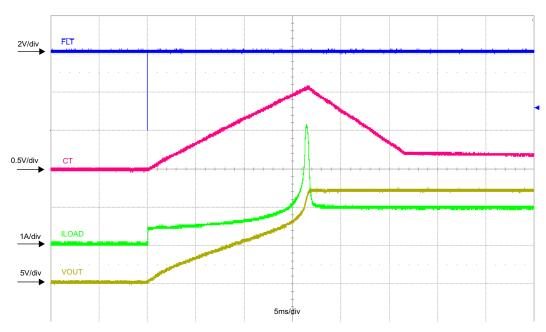
Figure 13. Fault Timer Operation During Startup
