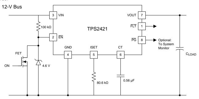
Figure 12. EN Delay Circuit
