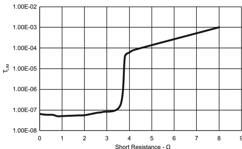
Figure 11. Overcurrent Response Time vs Short Resistance
