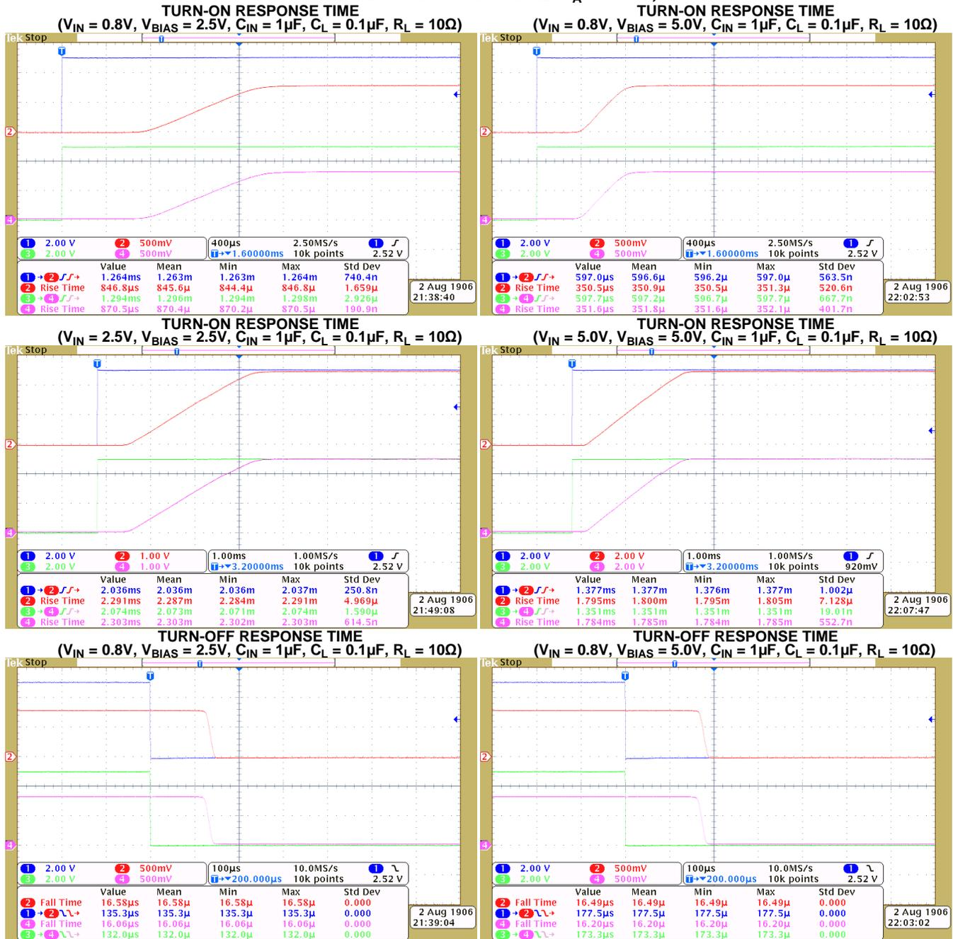
TYPICAL AC SCOPE CAPTURES @  $T_A = 25^\circ\text{C}$ ,  $C_T = 1\text{nF}$  (continued)
