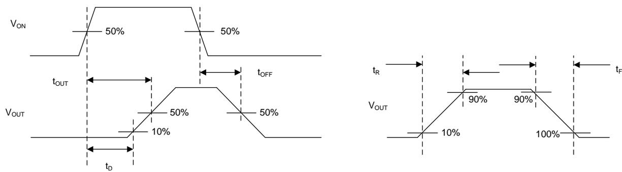
Figure 17. Timing Waveforms
