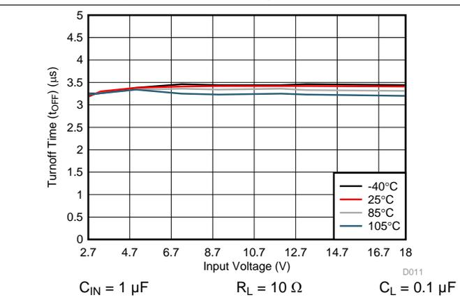
Figure 10. Turnoff Time ( $t_{OFF}$ ) vs Input Voltage
