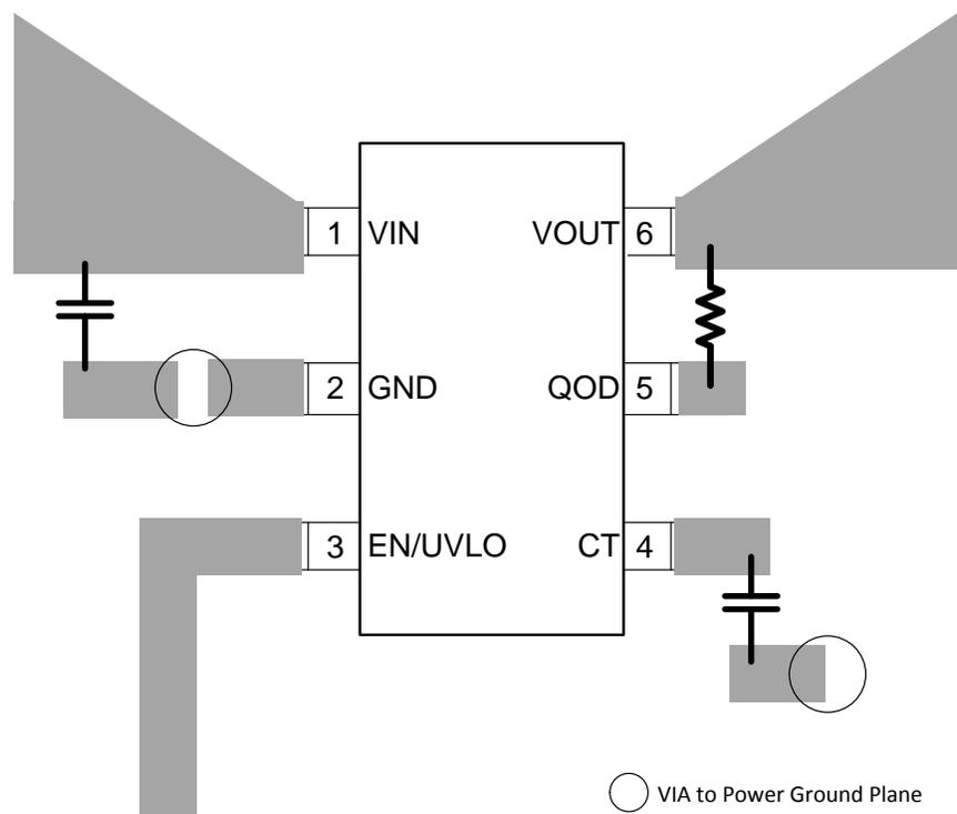
**Figure 34. Recommended Board Layout**
