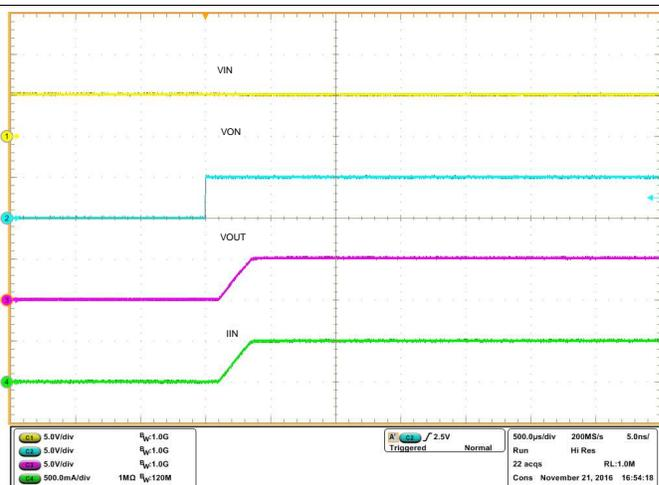
Figure 12. Rise Time  $t_R$  at  $V_{IN} = 5\text{ V}$
