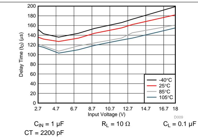
Figure 8. Delay Time ( $t_D$ ) vs Input Voltage
