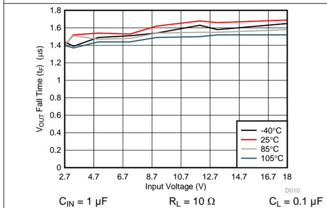
Figure 9.  $V_{OUT}$  Fall Time ( $t_F$ ) vs Input Voltage
