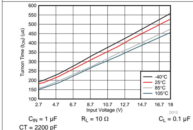
Figure 11. Turnon Time ( $t_{ON}$ ) vs Input Voltage
