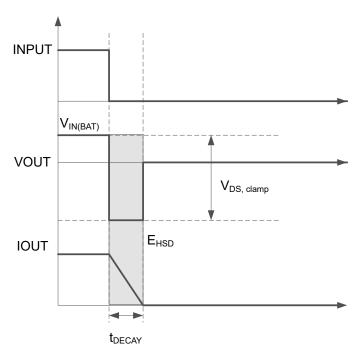
图 8-5. Inductive-Load Switching-Off Diagram
