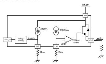
图 8-2. Current-Sense and Current-Limit Block Diagram
