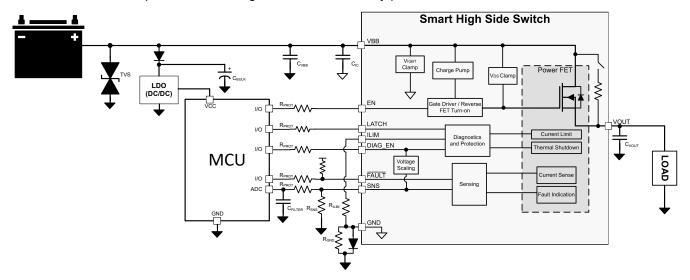
图 9-1. Typical Application Circuitry
