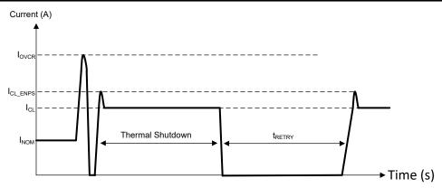
图 8-8. On-State Short-Circuit Behavior
