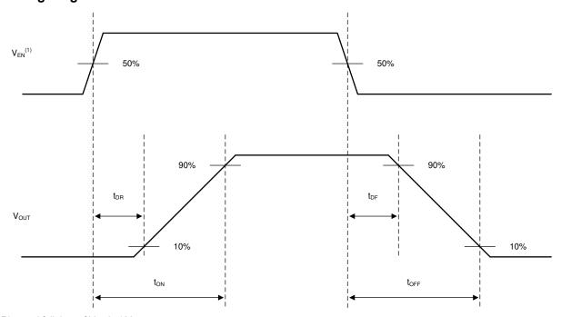
Rise and fall time of  $\ensuremath{V_{EN}}$  is 100 ns.
