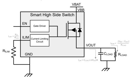
图 8-3. Capacitive Charging Circuit
