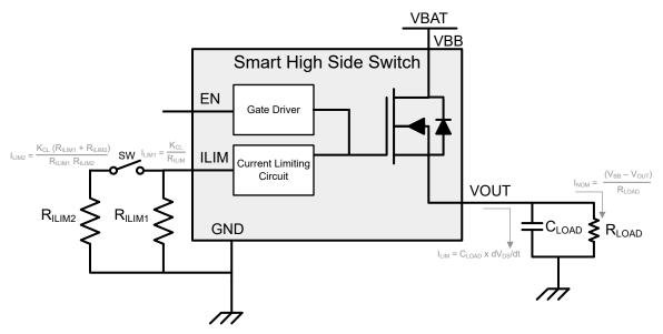
图 9-2. Dynamic Changing Current Limit Setup
