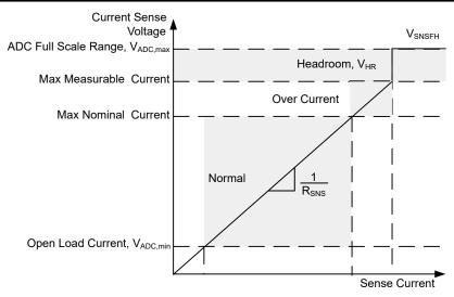
图 8-1. Voltage Indication on the Current-Sense Pin
