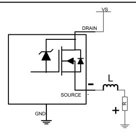
图 8-4. Driving Inductive Load
