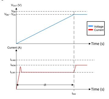
图 9-4. Large Capacitive Charging Changing Current Limit
