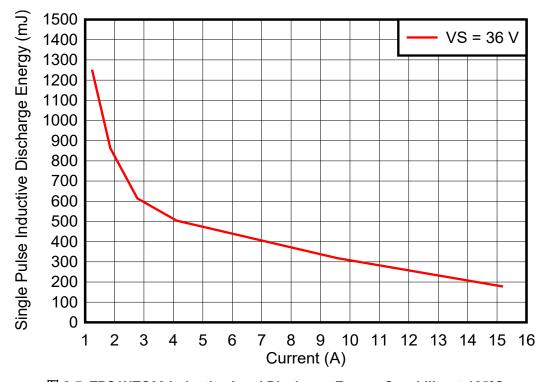
图 8-7. TPS1HTC30 Inductive Load Discharge Energy Capability at 125°C
