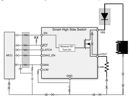
图 8-12. Reverse Protection With Blocking Diode
