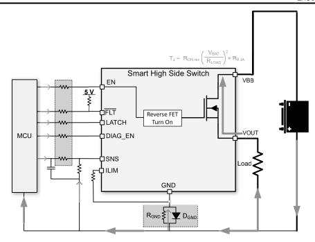
图 8-13. Reverse Protection With GND Network
