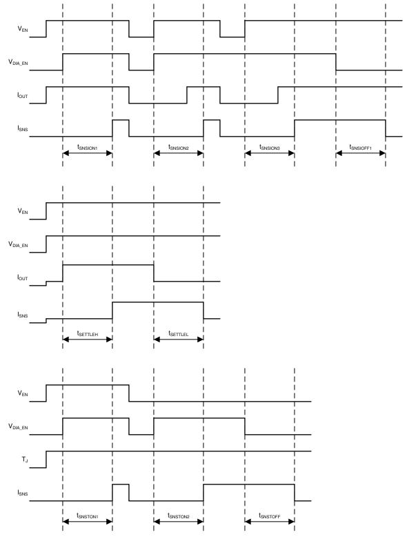
Rise and fall times of control signals are 100 ns. Control signals include: EN, DIA\_EN.
