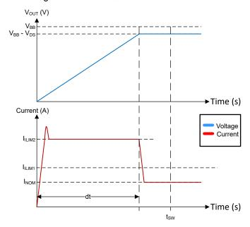
图 9-3. Capacitive Charging Changing Current Limit
