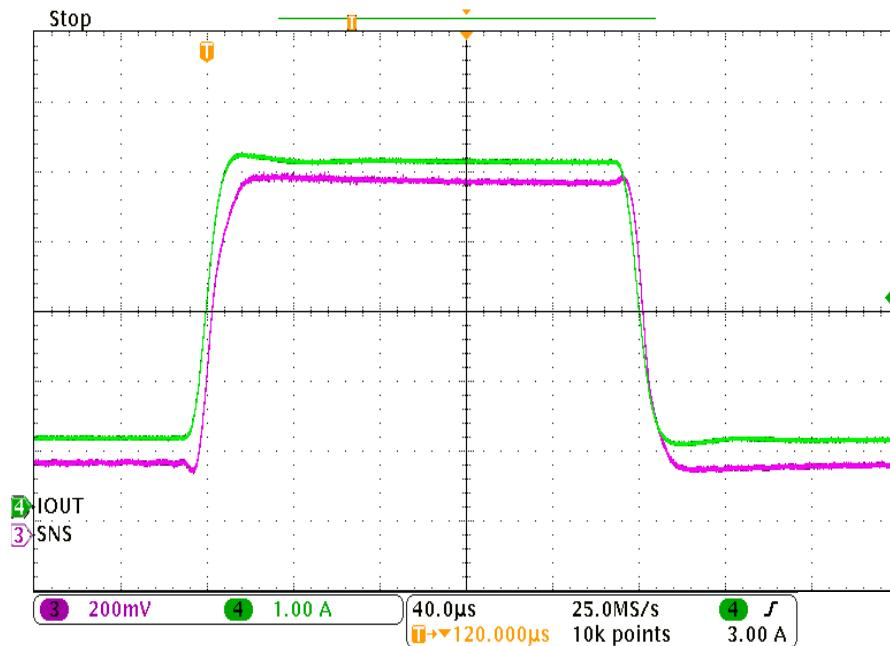
图 58. SNS Response During Heater Load Step
