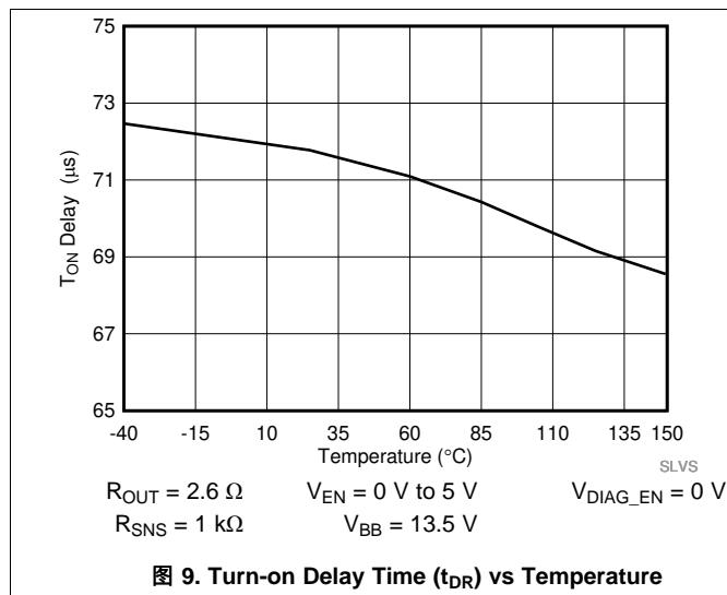
**图 9. Turn-on Delay Time ( $t_{DR}$ ) vs Temperature**
