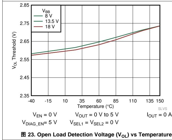
**图 23. Open Load Detection Voltage (V<sub>OL</sub>) vs Temperature**
