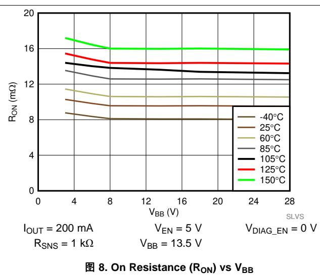
**图 8. On Resistance ( $R_{ON}$ ) vs  $V_{BB}$**
