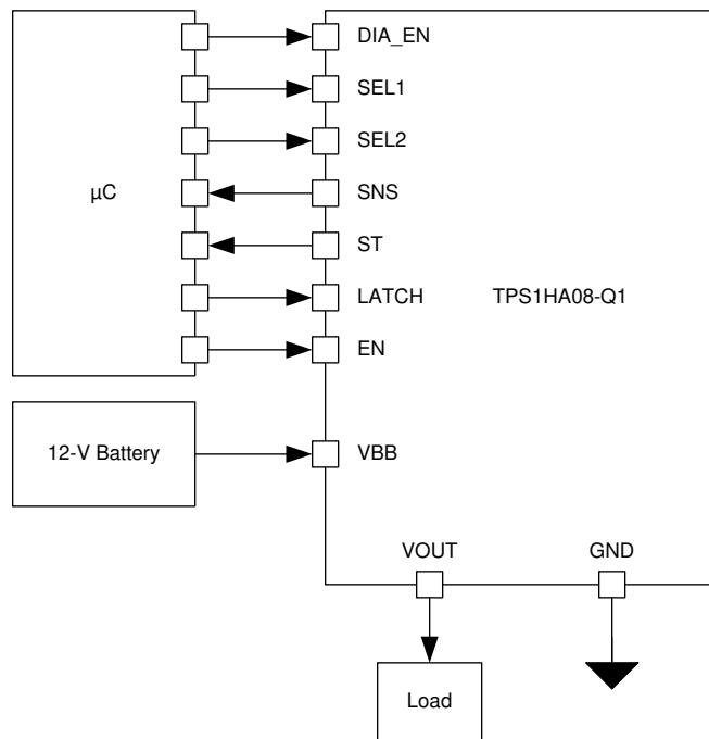
图 56. Block Diagram for Powering Heater Loads
