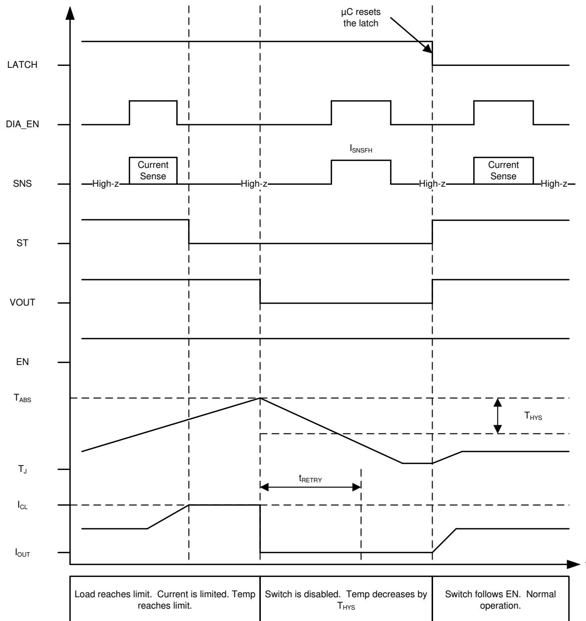
**图 44. Current Limit – Version C,D - Latched Behavior**
