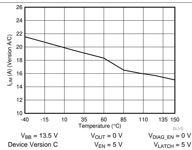
**图 22. Current Limit (I<sub>CL</sub>) vs Temperature**
