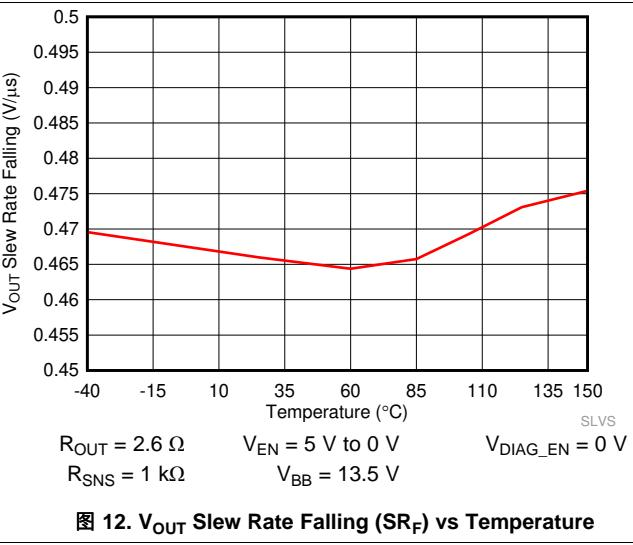
**图 12.  $V_{OUT}$  Slew Rate Falling ( $SR_F$ ) vs Temperature**
