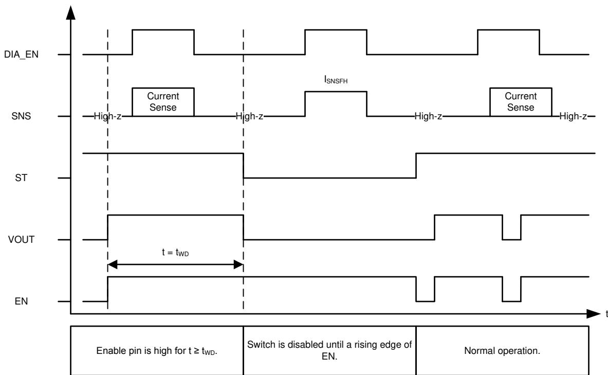
图 52. Enable Watchdog Timing Diagram
