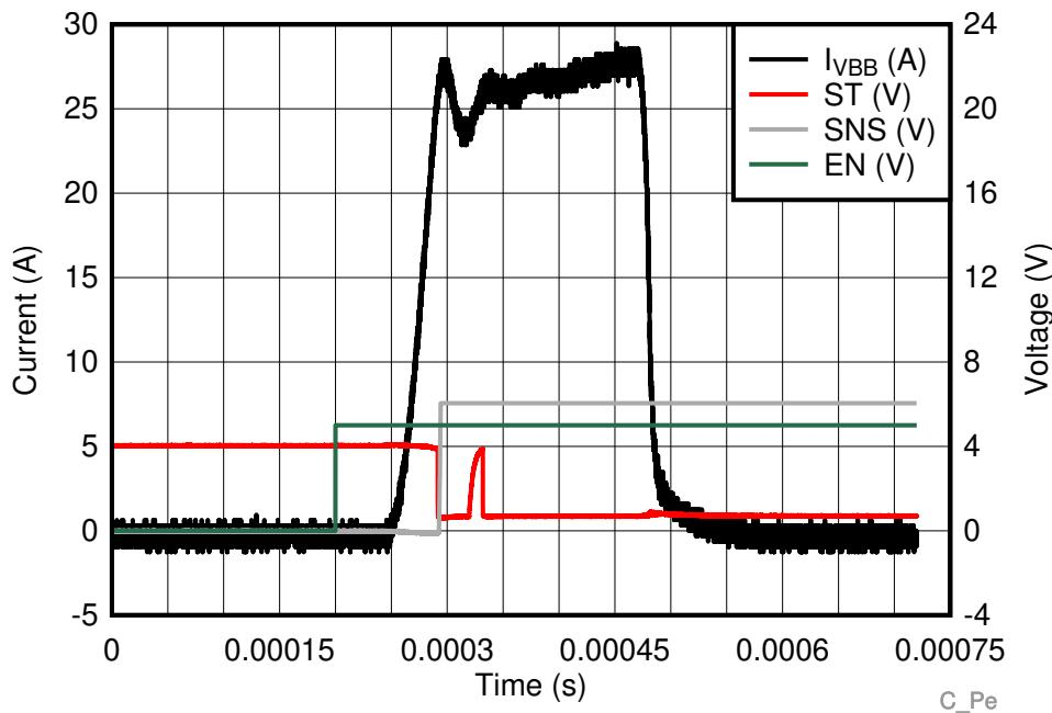
图 60. Overcurrent Behavior During Short Circuit Event
