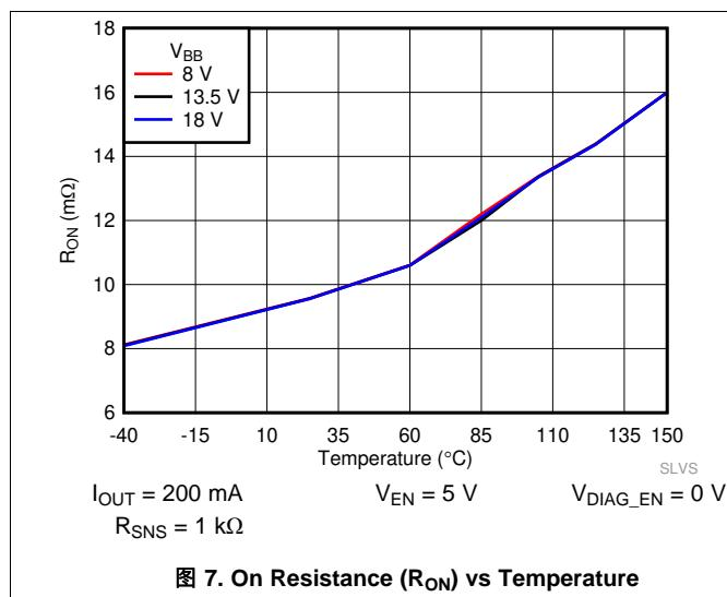
**图 7. On Resistance ( $R_{ON}$ ) vs Temperature**
