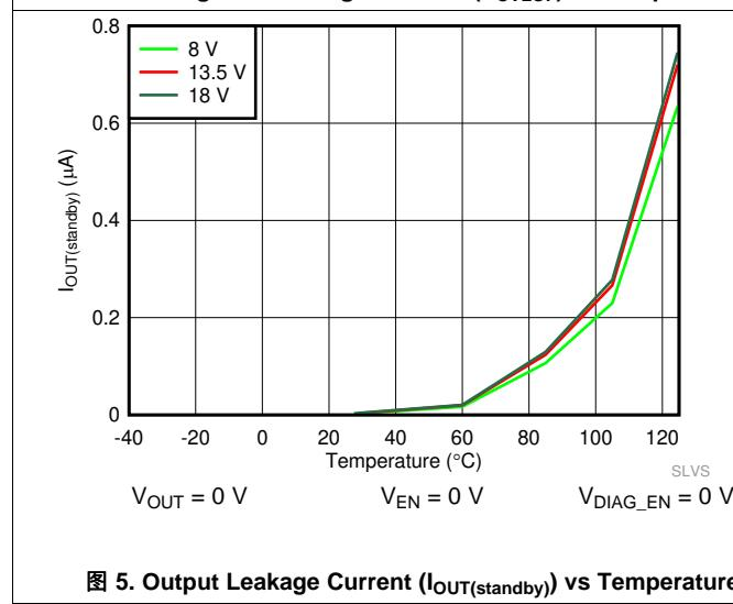
**图 5. Output Leakage Current ( $I_{OUT(standby)}$ ) vs Temperature**
