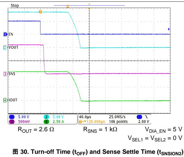
图 30. Turn-off Time ( $t_{OFF}$ ) and Sense Settle Time ( $t_{SENSETTLE}$ )
