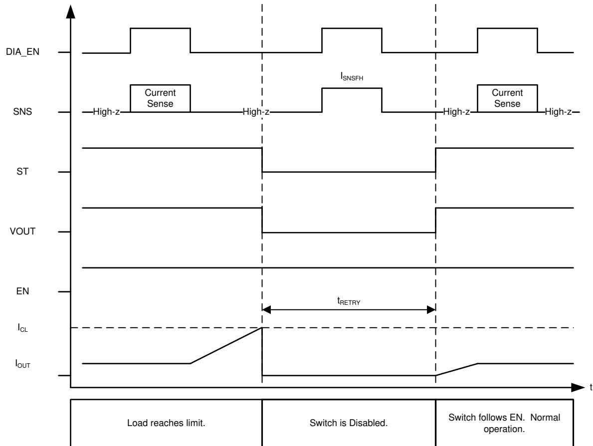
图 43. Current Limit – Version A,B,E - LATCH = 0
