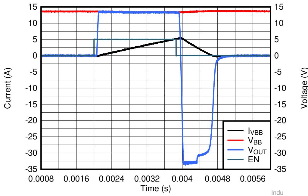
**图 40. Inductive Discharge (5 mH, 5 A)**
