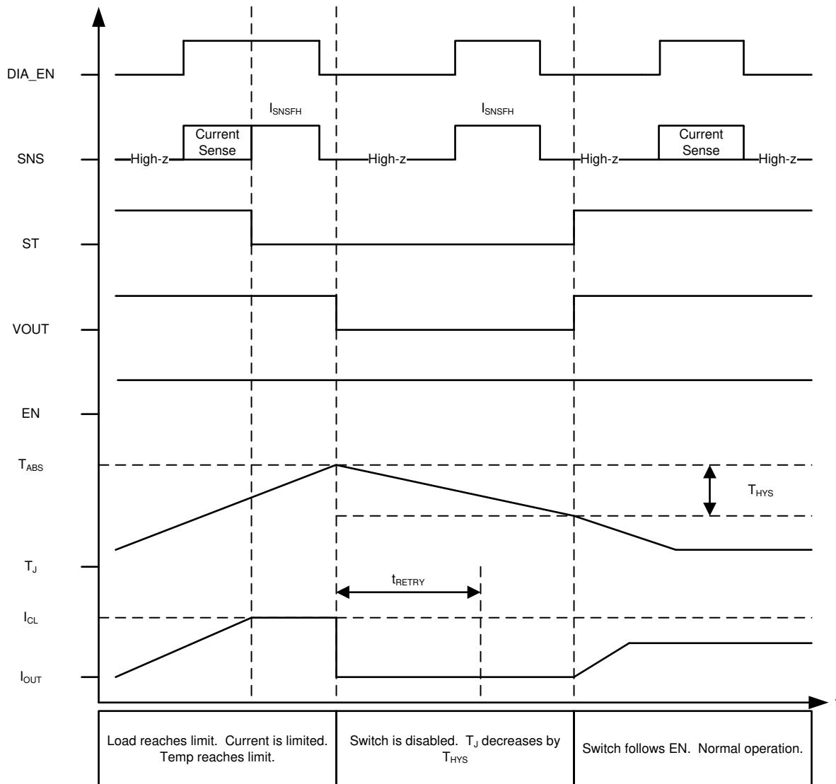
图 45. Current Limit – Version C,D - LATCH = 0
