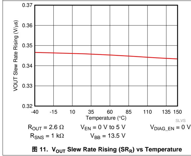
**图 11.  $V_{OUT}$  Slew Rate Rising ( $SR_R$ ) vs Temperature**
