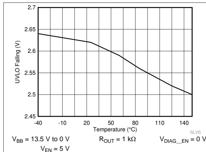
**图 3. Falling Undervoltage Lockout ( $V_{UVLOF}$ ) vs Temperature**
