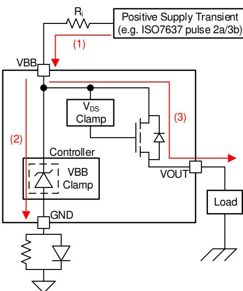
图 39. Current Path During Supply Voltage Transient
