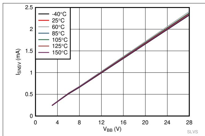
**图 19. Voltage Sense Output Current (I<sub>SNSV</sub>) vs V<sub>BB</sub>**
