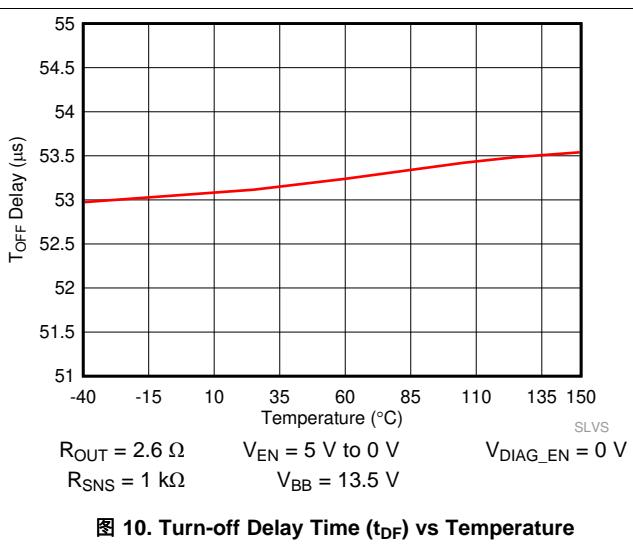
**图 10. Turn-off Delay Time ( $t_{DF}$ ) vs Temperature**
