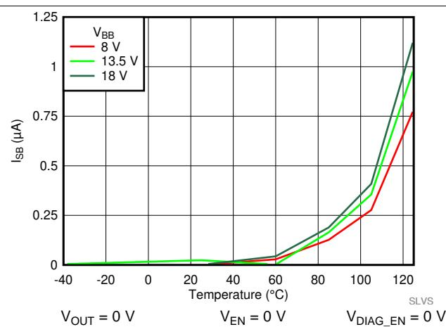
**图 4. Standby Current ( $I_{SB}$ ) vs Temperature**
