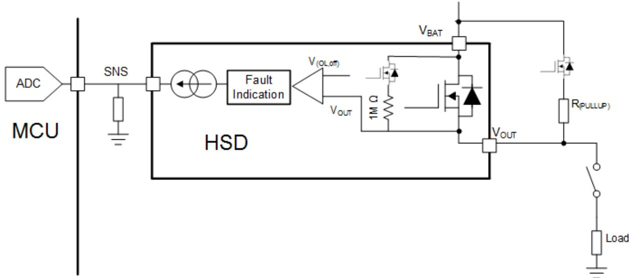
(1) This figure assumes that the device ground and the load ground are at the same potential. In application, there may be a ground shift voltage of 1 V to 2 V.
