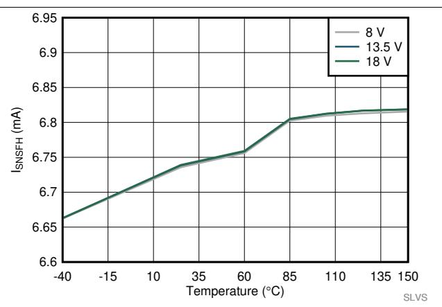
**图 20. Fault High Output Current (I<sub>SNSFH</sub>) vs Temperature**
