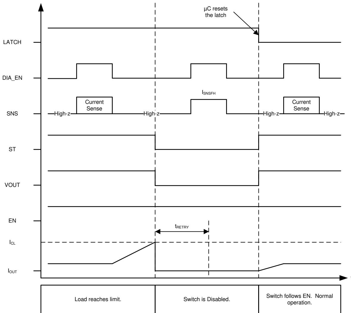
**图 42. Current Limit – Version A,B,E - Latched Behavior**
