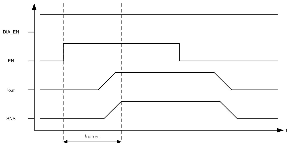
图 50. Current Sensing in Low-Duty Cycle Applications
