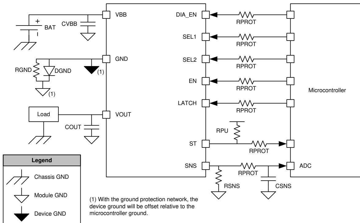
With the ground protection network, the device ground will be offset relative to the microcontroller ground.
