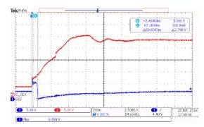
图 33. TPD6S300A Protecting the TPS65982 During a Short-to-V<sub>BUS</sub> Event
