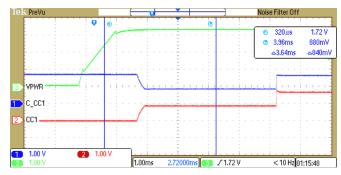
图 32. TPD6S300A Turning On in Dead Battery Mode with  $R_D$  on CC1
