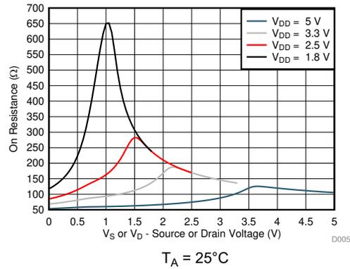
图 7-4. On-Resistance vs Source or Drain Voltage
