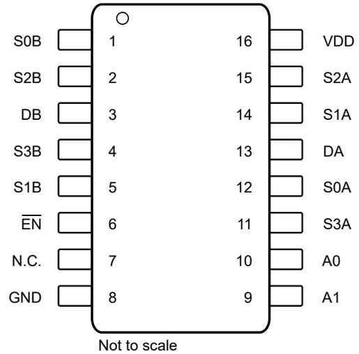
图 6-5. TMUX1309: DYY Package, 16-Pin SOT-23-THIN (Top View)
