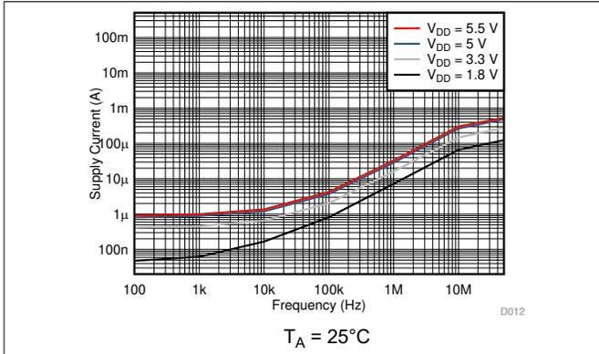
图 7-7. Supply Current vs Input Switching Frequency
