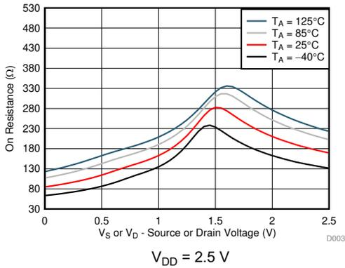
图 7-3. On-Resistance vs Temperature
