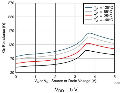
图 7-1. On-Resistance vs Temperature
