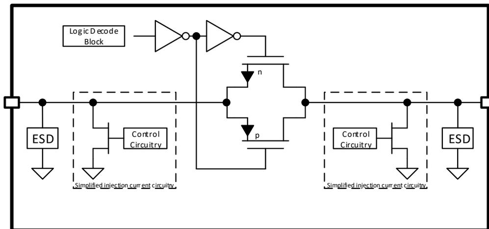
图 9-3. Simplified Diagram of Injection Current Control
