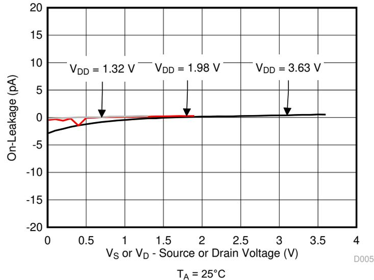
图 9-5. On-Leakage vs Source or Drain Voltage
