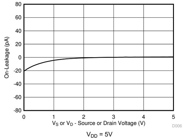
图 9-3. On-Leakage vs Source or Drain Voltage
