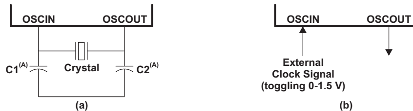
Figure 5-5. Recommended Crystal/Clock Connection
