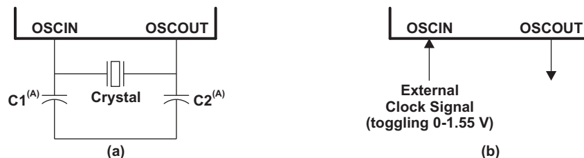
Figure 5-3. Recommended Crystal/Clock Connection
