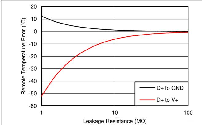
图 6-4. Remote Temperature Error vs. Leakage Resistance
