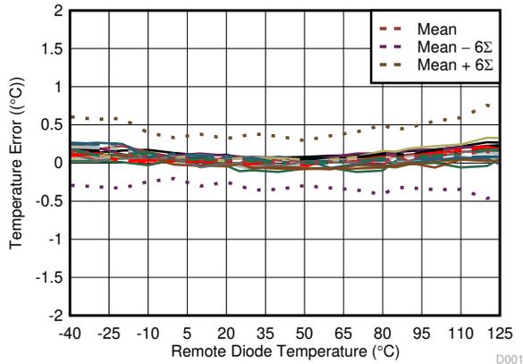
图 8-3. TMP451-Q1 Remote Diode Temperature Drift (Diode-Connected 2N3906)
