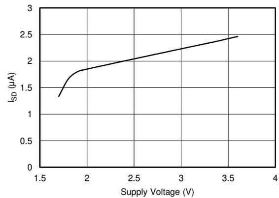
图 6-11. Shutdown Quiescent Current vs. Supply Voltage
