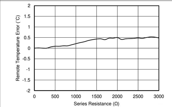
图 6-5. Remote Temperature Error vs. Series Resistance
