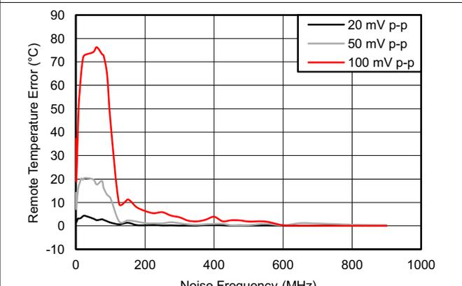
图 6-7. Remote Temperature Error vs. Remote Channel Noise Frequency
