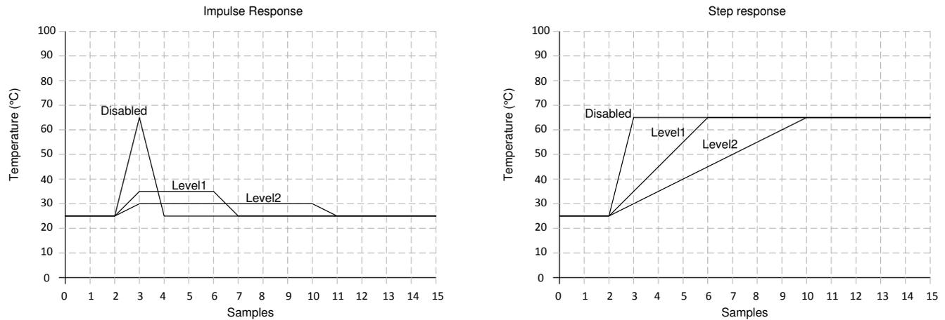
**图 7-1. Filter Response to Impulse and Step Inputs**
