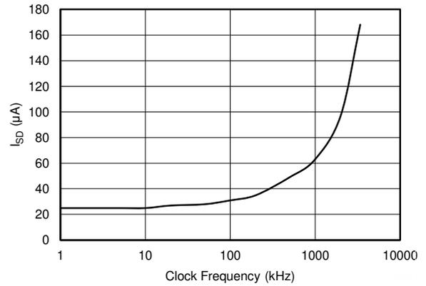
图 6-9. Shutdown Quiescent Current vs. SCL Clock Frequency
