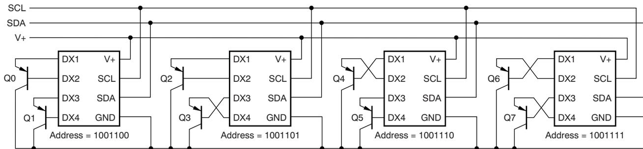
**Figure 18. TMP422-Q1 Connections for Device Address Setup**
