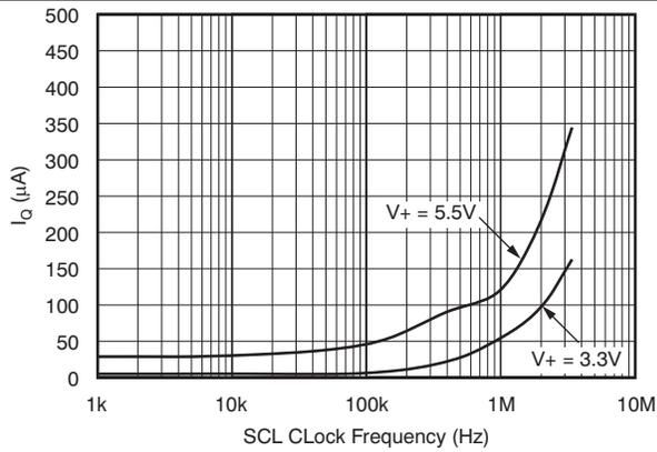
**Figure 10. Shutdown Quiescent Current vs SCL Clock Frequency**
