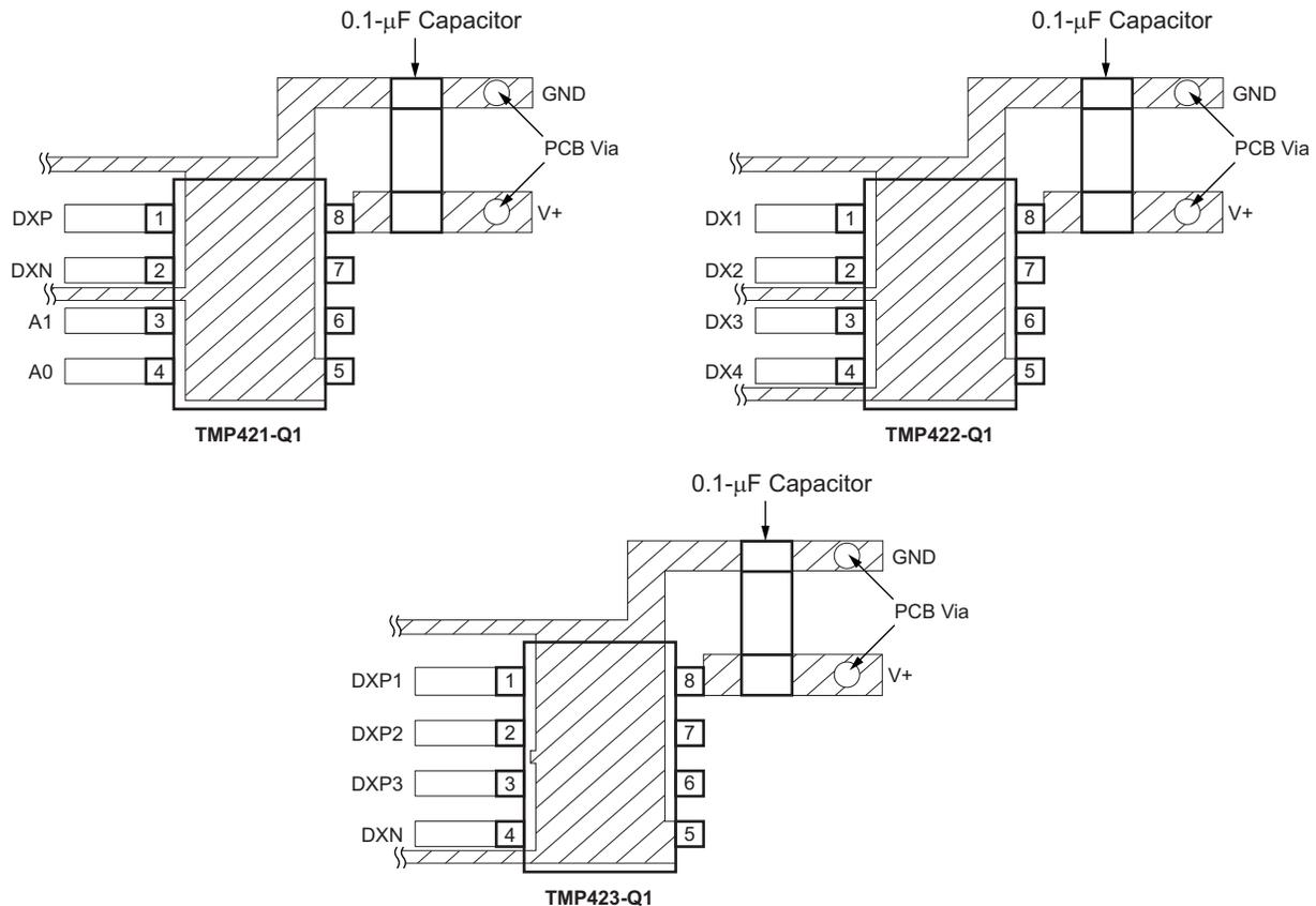
**Figure 24. Suggested Bypass Capacitor Placement and Trace Shielding**
