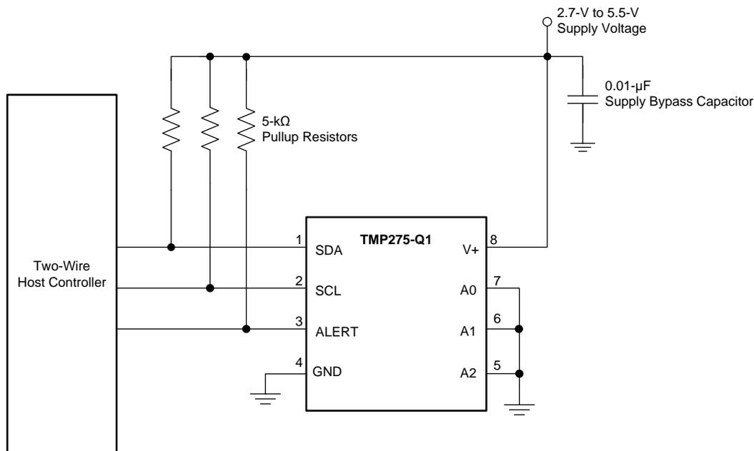
Figure 13. Typical Connections of the TMP275-Q1 Schematic
