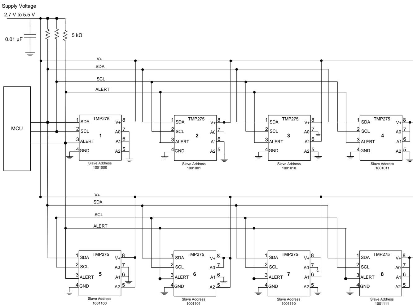
Figure 15. Connecting Multiple Devices on a Single Bus
