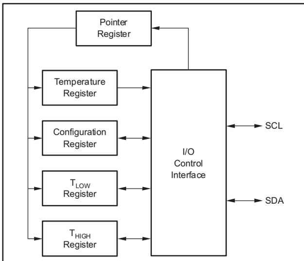
**Figure 11. Internal Register Structure of the TMP275-Q1**
