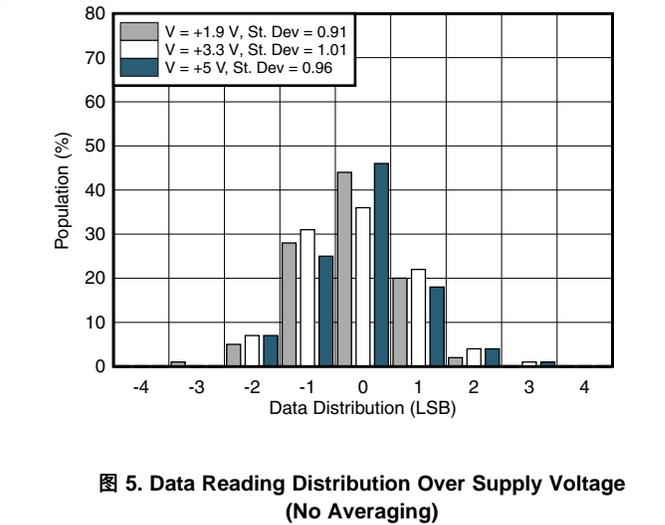
图 5. Data Reading Distribution Over Supply Voltage (No Averaging)
