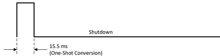
**图 21. One-Shot Timing Diagram With No Averaging**
