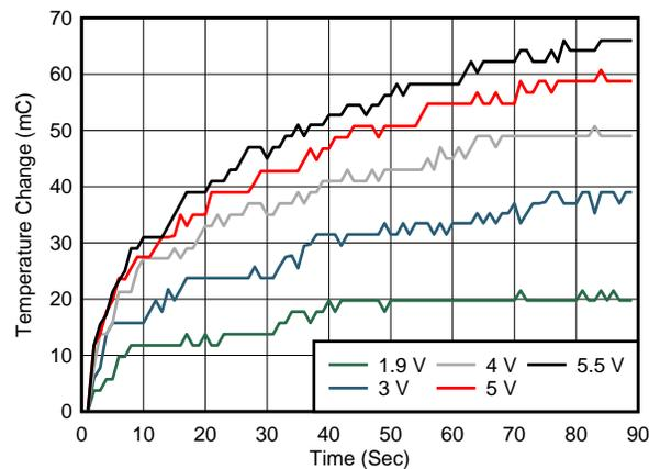
图 42. Self-Heating in Still Air vs. Temperature and Dissipated Power
