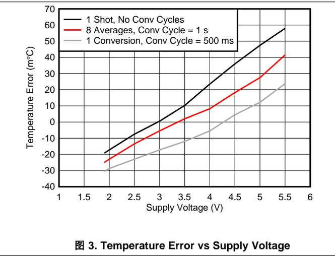
图 3. Temperature Error vs Supply Voltage
