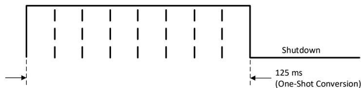
**图 22. One-Shot Timing Diagram With 8 Averages**
