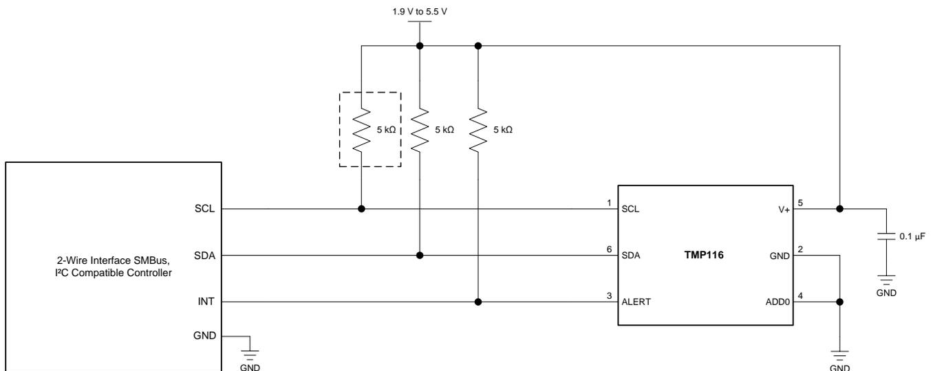
NOTE: The SDA and ALERT pins require pullup resistors.
