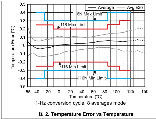
图 2. Temperature Error vs Temperature
