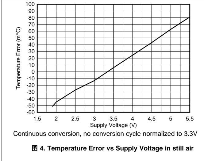
图 4. Temperature Error vs Supply Voltage in still air
