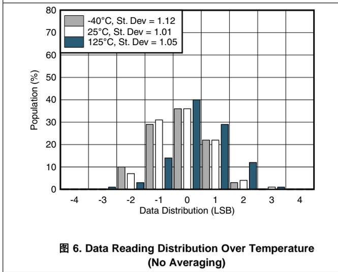
图 6. Data Reading Distribution Over Temperature (No Averaging)
