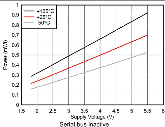
图 12. Power Consumption During Active Conversion
