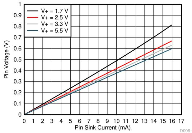
图 8-8. ALERT Pin Output Voltage vs. Sink Current
