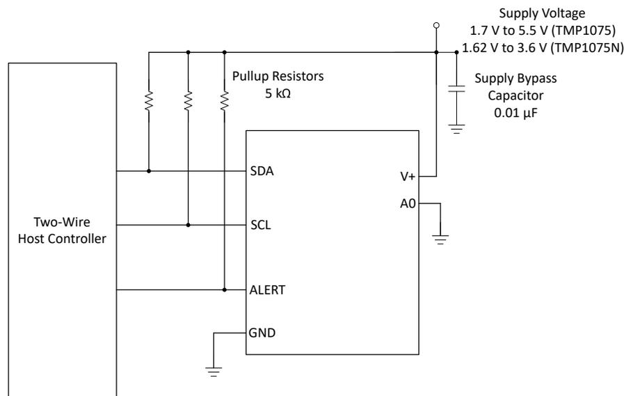
图 10-1. Typical Connections
