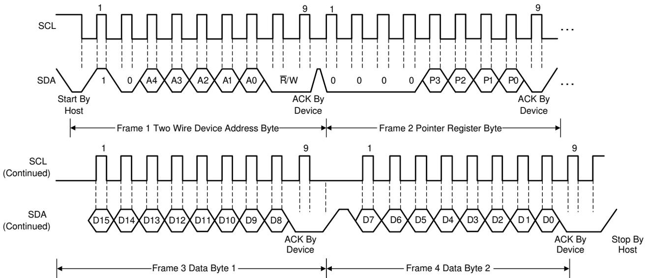
图 9-3. Two-Wire Timing Diagram for Write Word Format
