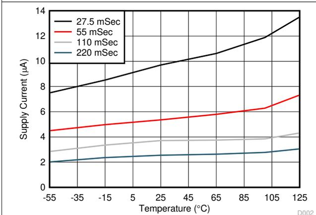
**图 8-5. Average Current vs. Conversion Rates and Temperature**
