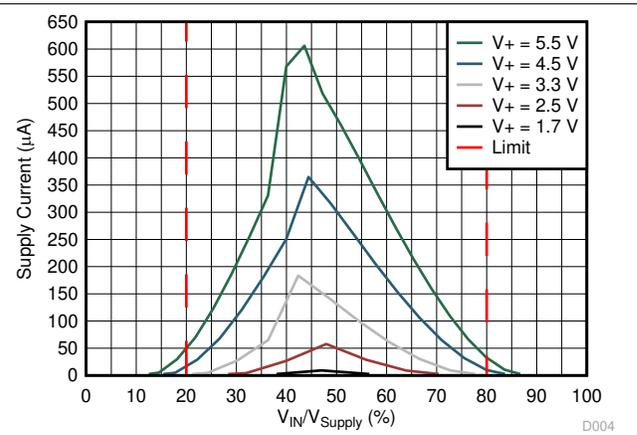
**图 8-6. Supply Current vs. Input Cell Voltage**
