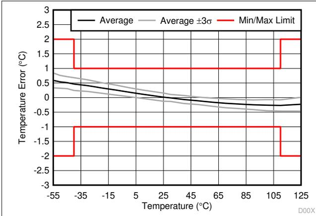
**图 8-1. DGK & D Temperature Error vs. Temperature**
