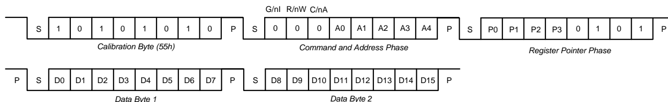
Figure 26. Individual Write Operation
