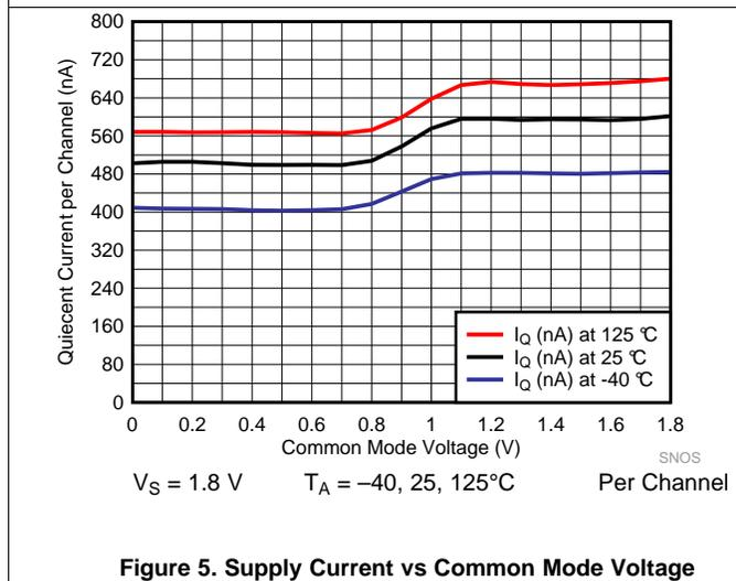
Figure 5. Supply Current vs Common Mode Voltage
