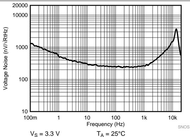
Figure 23. Input Voltage Noise vs Frequency
