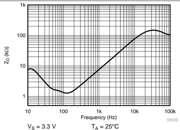
Figure 24. Open Loop Output Impedance
