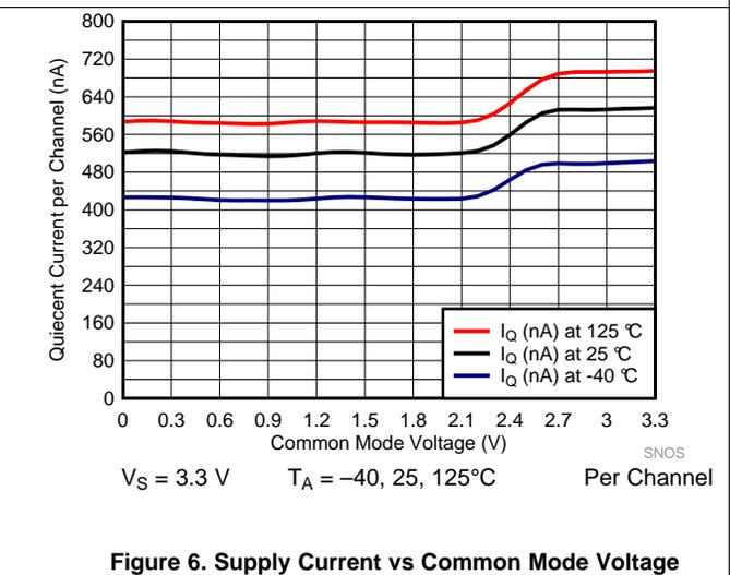
Figure 6. Supply Current vs Common Mode Voltage
