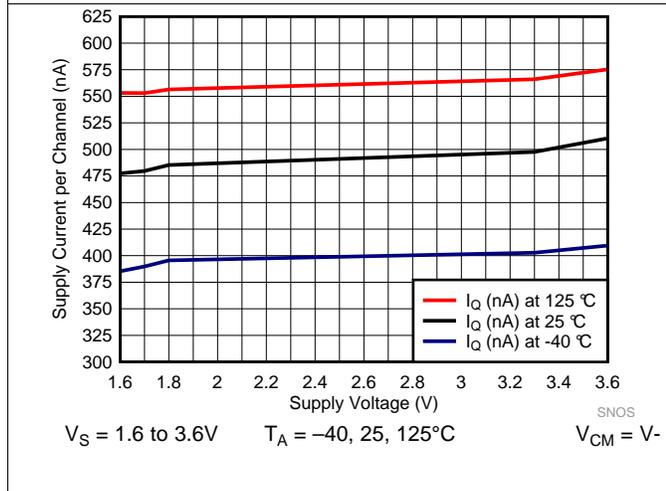
Figure 9. Supply Current vs Supply Voltage, Low VCM
