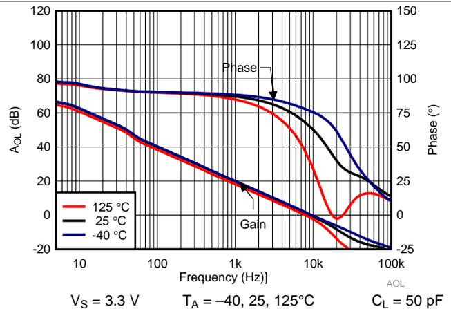
Figure 22. Open Loop Gain and Phase
