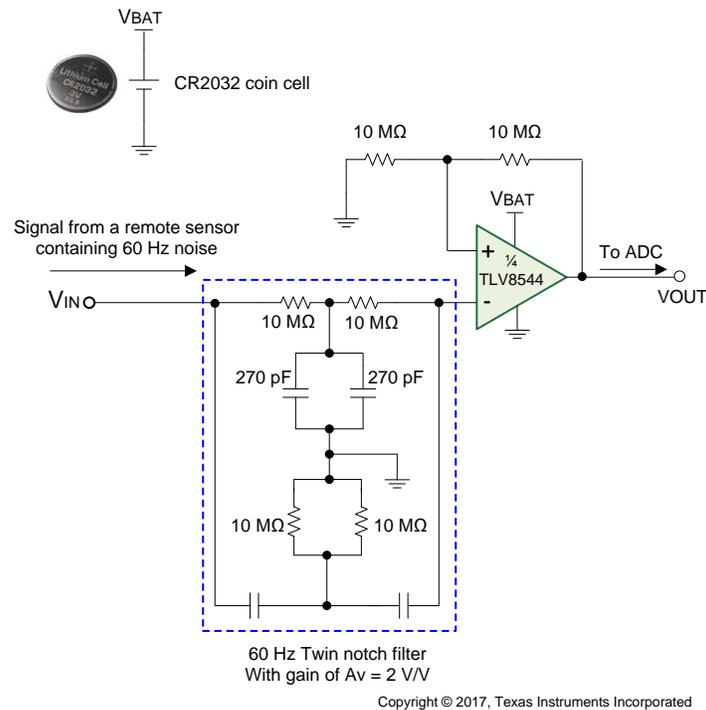
**Figure 36. 60 Hz-Notch Filter**
