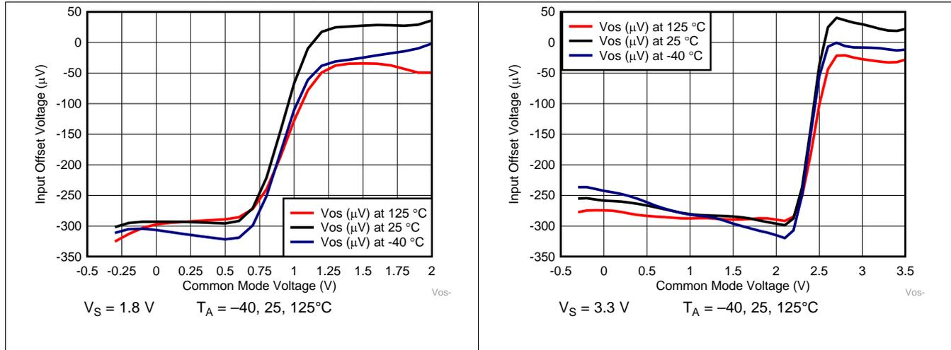
Figure 7. Typical Offset Voltage vs Common Mode Voltage
