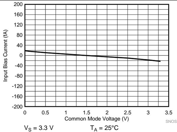
Figure 19. Input Bias Current vs Common Mode Voltage
