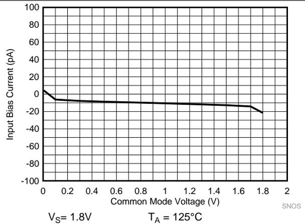
Figure 20. Input Bias Current vs Common Mode Voltage
