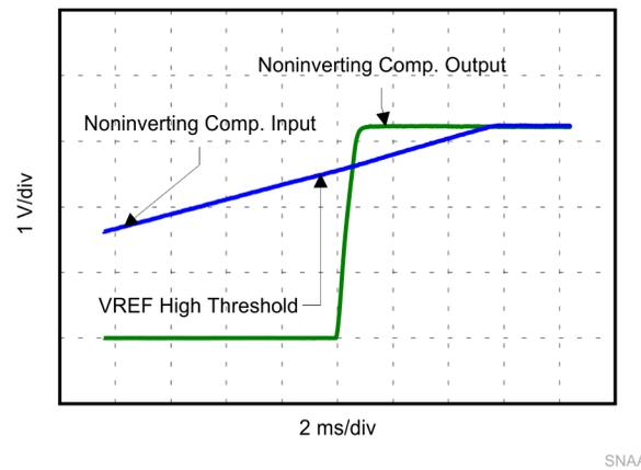
**Figure 34. Noninverting Comparator Input and Output Signals**
