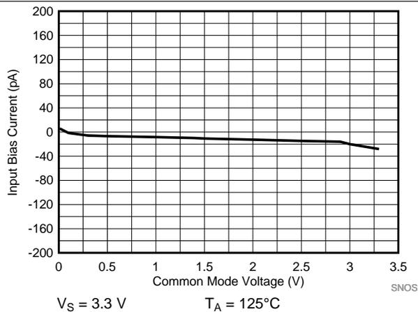
Figure 21. Input Bias Current vs Common Mode Voltage
