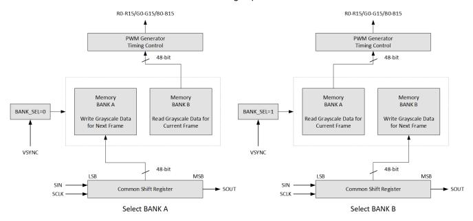
图 8-26. Bank Selection Exchange Operation
