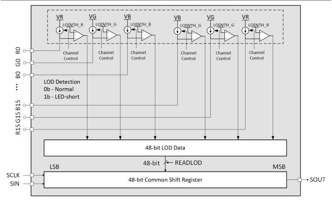
图 8-8. LED Open Detection Circuit
