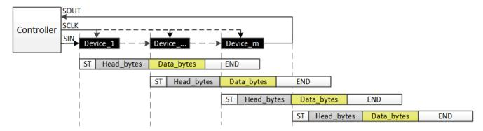
图 8-21. Data Write Command with Broadcast
