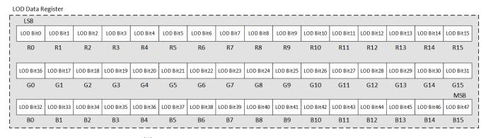
图 8-9. Bit Arrangement in LOD Data Register
