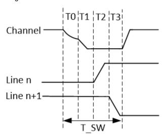
图 8-7. Line Transitioning Sequence
