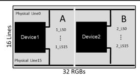
图 8-1. Two Devices in Independent Mode
