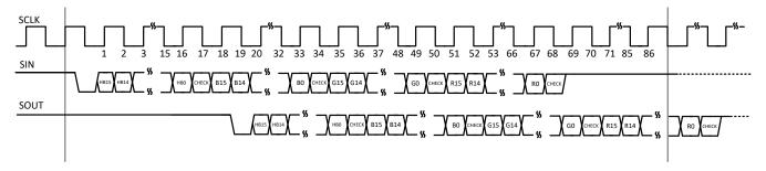
图 8-22. Data Write Command with Broadcast (Timing Diagram)
