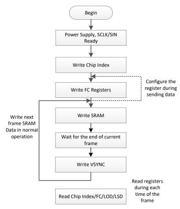
图 9-3. Design Procedure for LED Display
