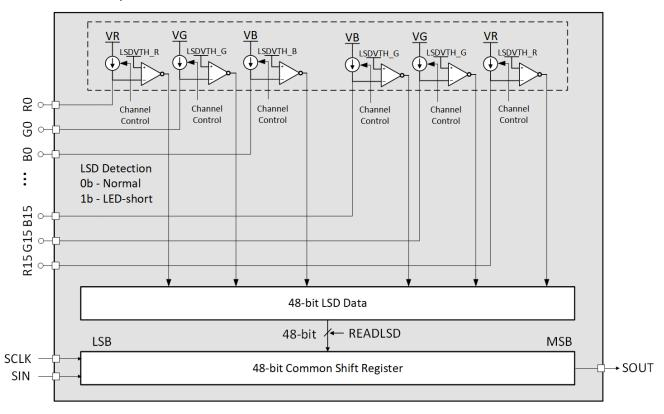
图 8-12. LED Short Detection Circuit
