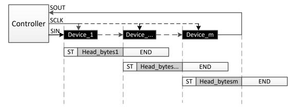
图 8-18. Chip Index Write Command
