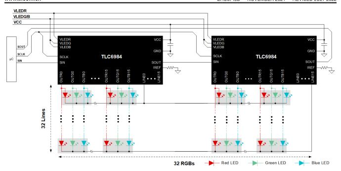
图 9-1. TLC6984 With Dual Devices Stackable Connection
