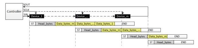
图 8-23. Data Write Command with Non-Broadcast
