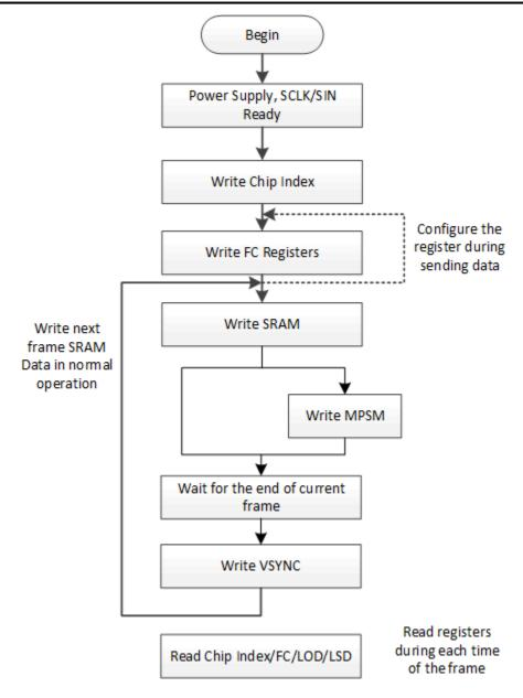
图 8-20. Design Procedure for MPSM Command
