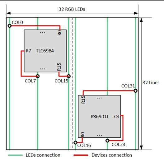
图 11-4. Channel Routing Suggestion With Channel Order Sequence
