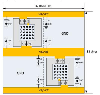
图 11-1. Power Rails Routing Suggestion
