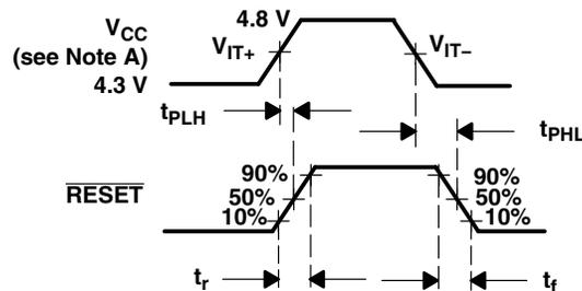
NOTE A:  $V_{CC}$  slew rate  $\leq 5 \mu\text{s}$
