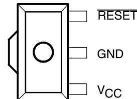
GND is in electrical contact with the tab.
