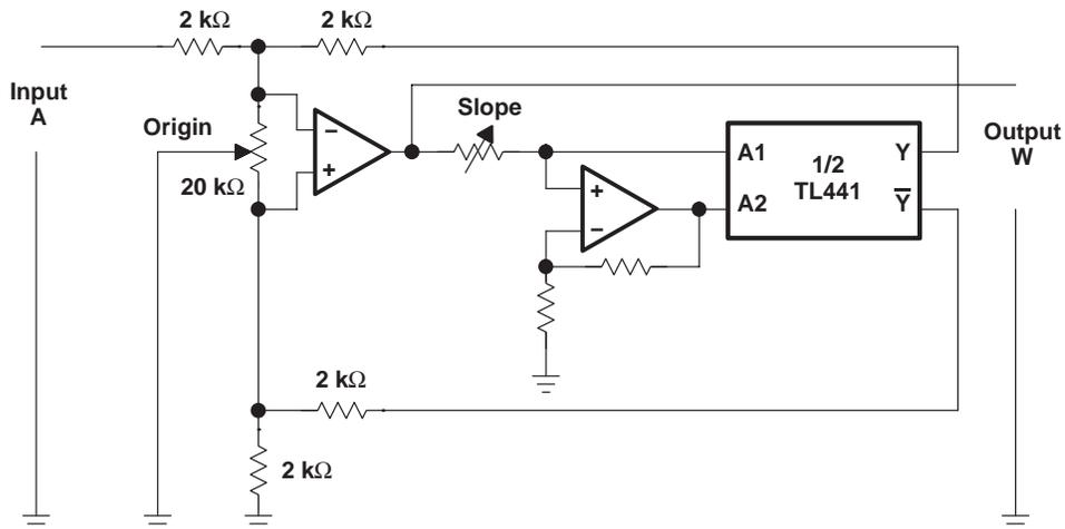
NOTE: Adjust the slope to correspond to the base "a". Exponential to any base:  $W = a$ .
