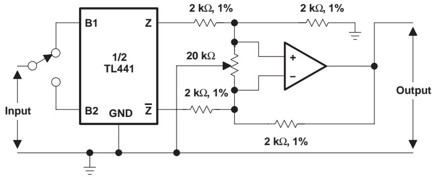
Figure 12. Utilization of Separate Stages
