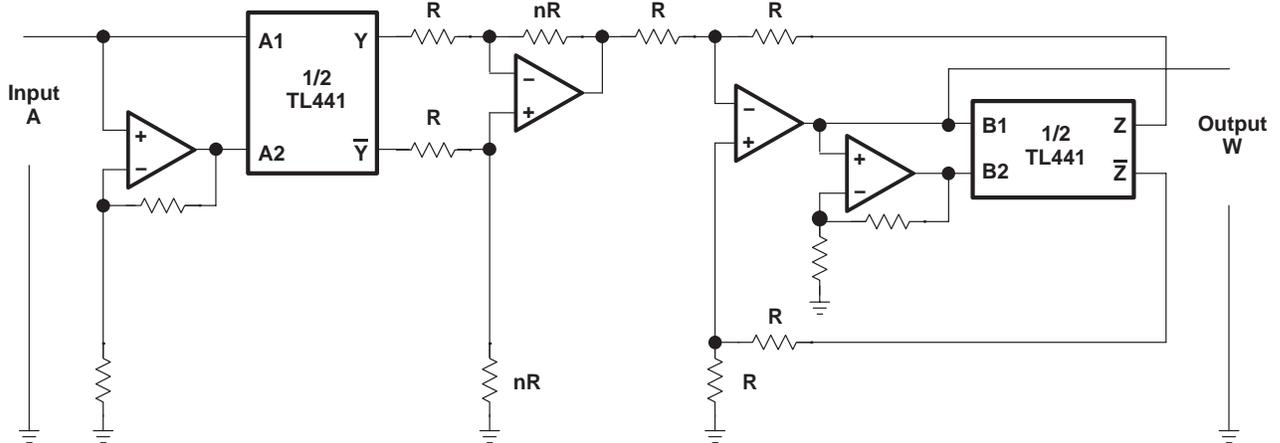
NOTE: R designates resistors of equal value, typically 2 k $\Omega$  to 10 k $\Omega$ . The power to which the input variable is raised is fixed by setting nR.
