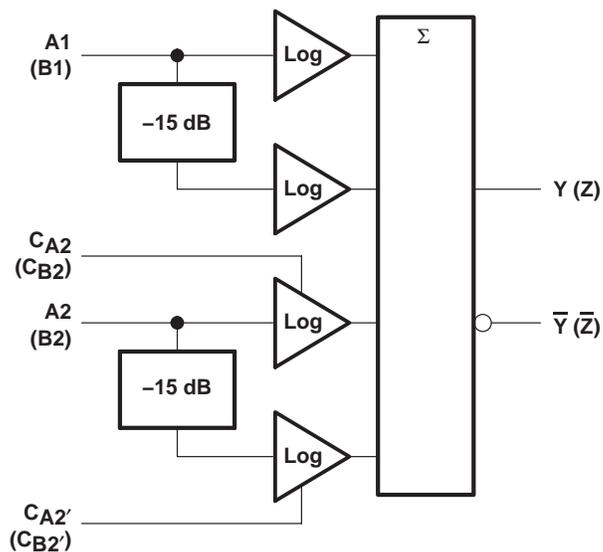
$Y \propto \log A1 + \log A2$ ;  $Z \propto \log B1 + \log B2$  where: A1, A2, B1, and B2 are in dBV, 0 dBV = 1 V.
