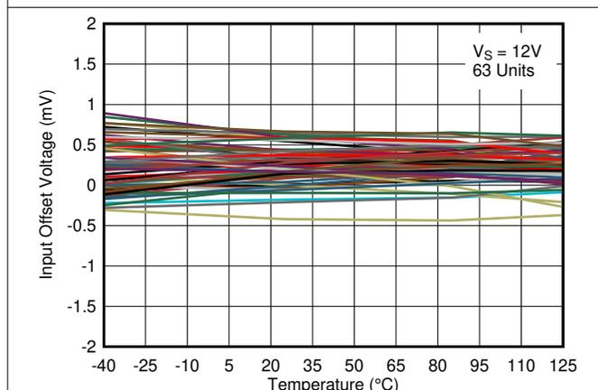
图 5-17. Input Offset Voltage vs. Temperature at 12V
