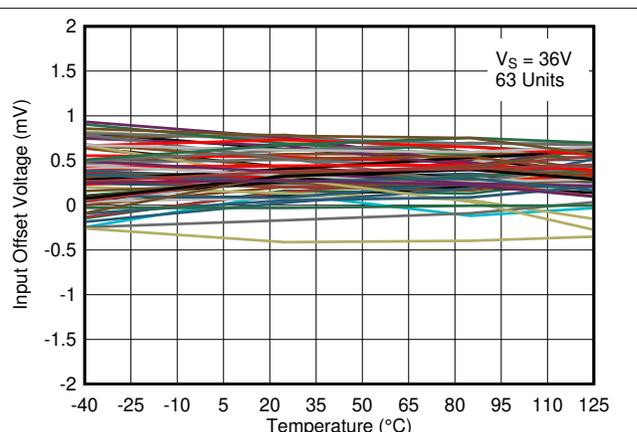
图 5-18. Input Offset Voltage vs. Temperature at 36V
