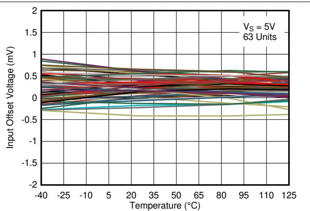
图 5-16. Input Offset Voltage vs. Temperature at 5V
