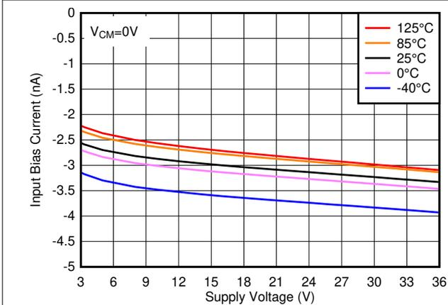
图 5-7. Input Bias Current vs. Supply Voltage
