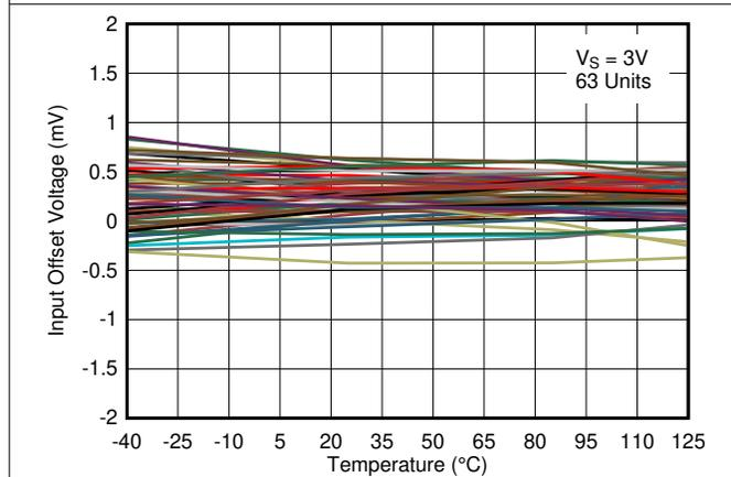
图 5-15. Input Offset Voltage vs. Temperature at 3V
