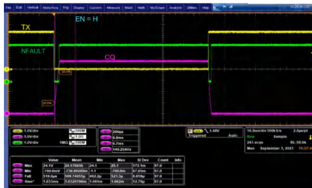
NFAULT is indicated for the duration of charging and discharging of the capacitor but driver is not disabled when ILIM_ADJ is floating L+ = 24\text{ V} C_L = 20\ \mu\text{F} R_L = 100\ \Omega R_{SET} = 1\text{ M}\Omega (ILIM_ADJ Floating) T_A = 25\text{ }^\circ\text{C}
