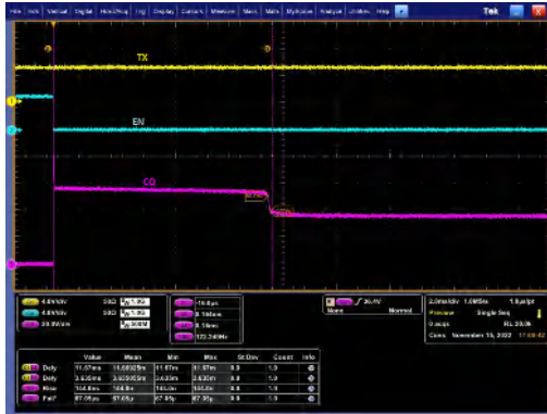
L+ = 36\text{ V} L = 1.5\text{ H} R_L = 360\ \Omega R_{SET} = 10\text{ k}\Omega T_A = 25\text{ }^\circ\text{C}
