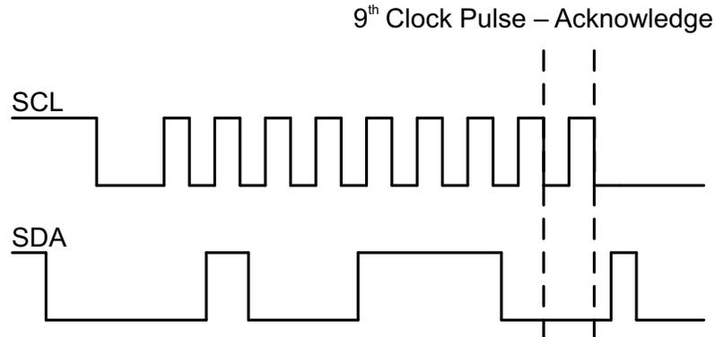
图 6-1. Bus A (0.8V to 5.5V Bus) Waveform
