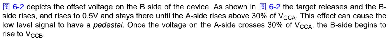
Figure 6-2 depicts the offset voltage on the B side of the device. As shown in Figure 6-2 the target releases and the B-side rises, and rises to 0.5V and stays there until the A-side rises above 30% of  $V_{CCA}$ . This effect can cause the low level signal to have a *pedestal*. Once the voltage on the A-side crosses 30% of  $V_{CCA}$ , the B-side begins to rise to  $V_{CCB}$ .
