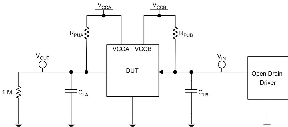
图 6-2. Test Circuit for Open-Drain Output from B to A
