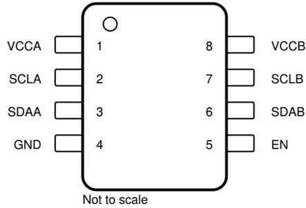
**图 4-1. DGK Package, 8-Pin VSSOP (Top View)**
