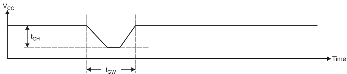
Figure 9. Glitch Width and Glitch Height
