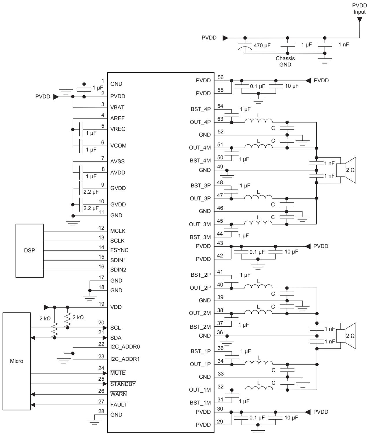
图 62. TAS6424L-Q1 Typical 2-Channel PBTB Application Schematic
