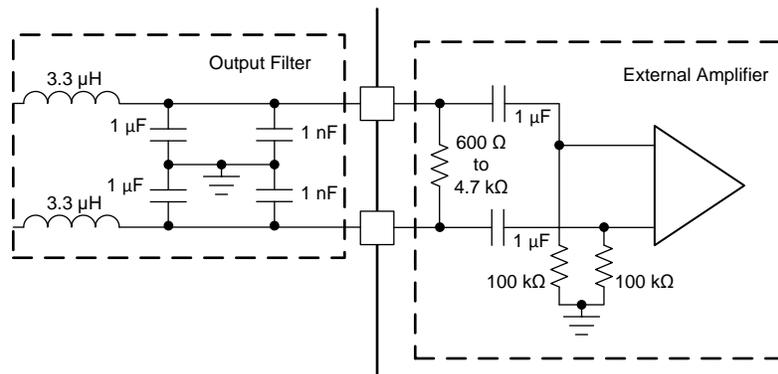
图 58. External Amplifier Input Configuration for Line Driver
