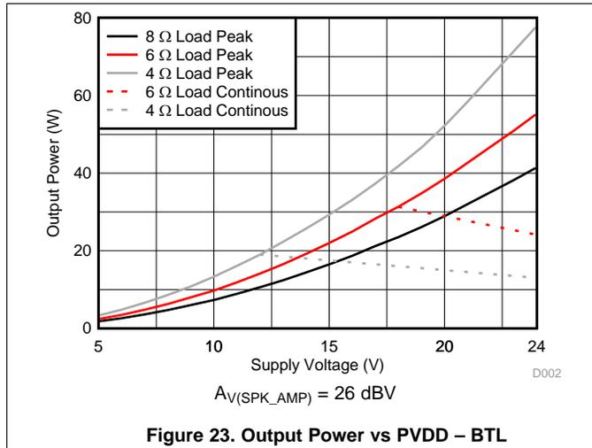
Figure 23. Output Power vs PVDD – BTL
