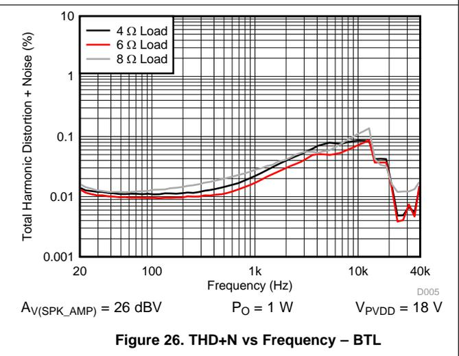
Figure 26. THD+N vs Frequency – BTL
