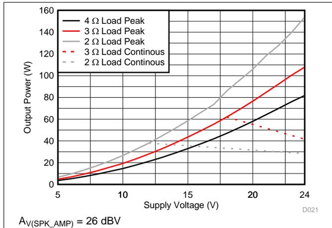
Figure 43. Output Power vs PVDD – PBTL
