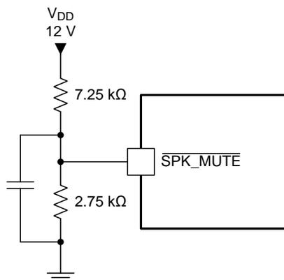
**Figure 66.  $\overline{\text{SPK\_MUTE}}$  Used in External Undervoltage Error Protection**
