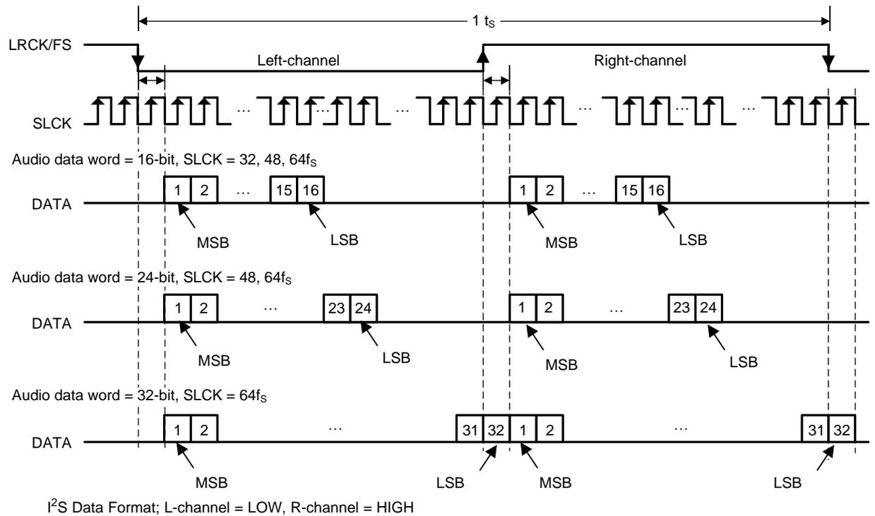
Figure 61. I<sup>2</sup>S Audio Data Format
