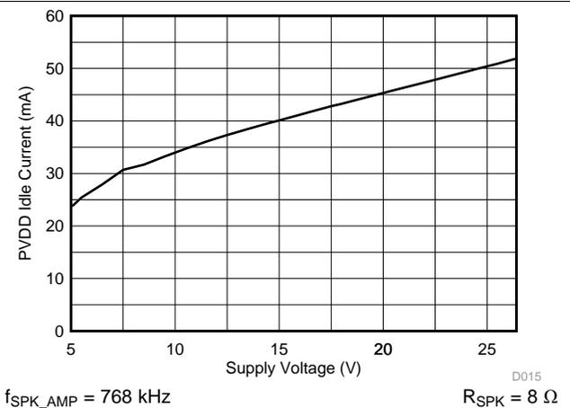
Figure 36. Idle Current Draw (Filterless) vs  $V_{PVDD}$  – BTL
