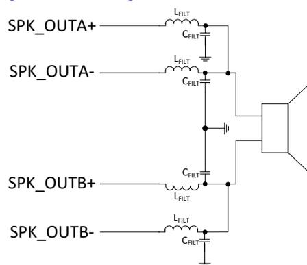
**Figure 71. Post-Filter PBTL**
