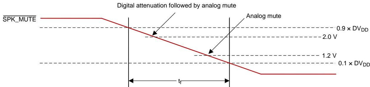
Figure 67. SPK\_MUTE Timing for External Undervoltage Error Protection
