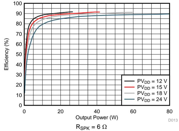
Figure 34. Efficiency vs Output Power – BTL
