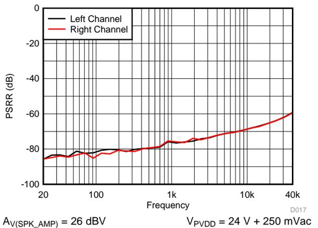
Figure 38. PVDD PSRR vs Frequency – BTL
