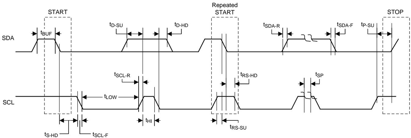
Figure 21. I<sup>2</sup>C Communication Port Timing Diagram
