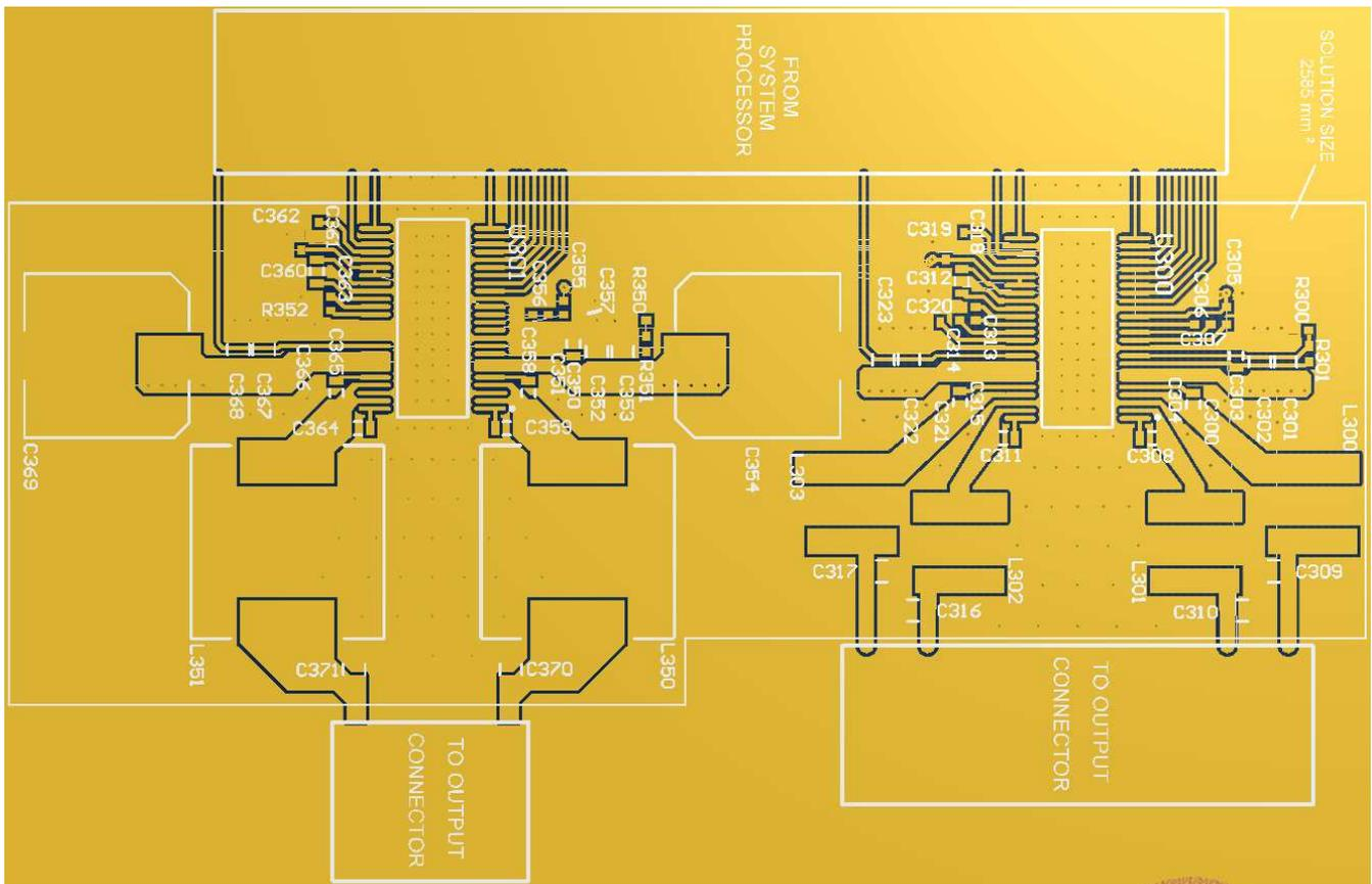
图 93. 2.1 (Stereo BTL + Mono PBTL) Top Copper View
