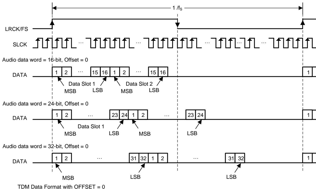
In TDM Modes, Duty Cycle of LRCK/Fs should be 1x SCLK at minimum. Rising edge is considered frame start.
