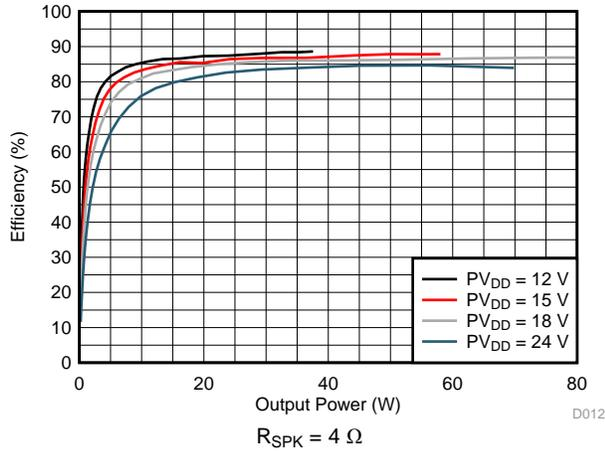
Figure 33. Efficiency vs Output Power – BTL
