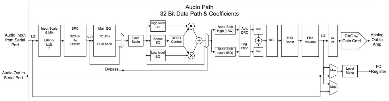
Figure 72. Fixed-Function Process Flow found in the TAS5780M
