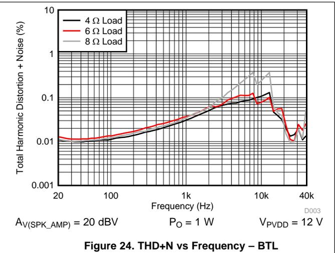
Figure 24. THD+N vs Frequency – BTL
