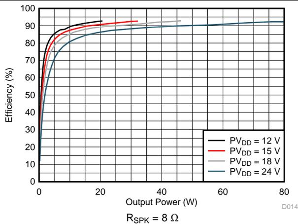
Figure 35. Efficiency vs Output Power – BTL
