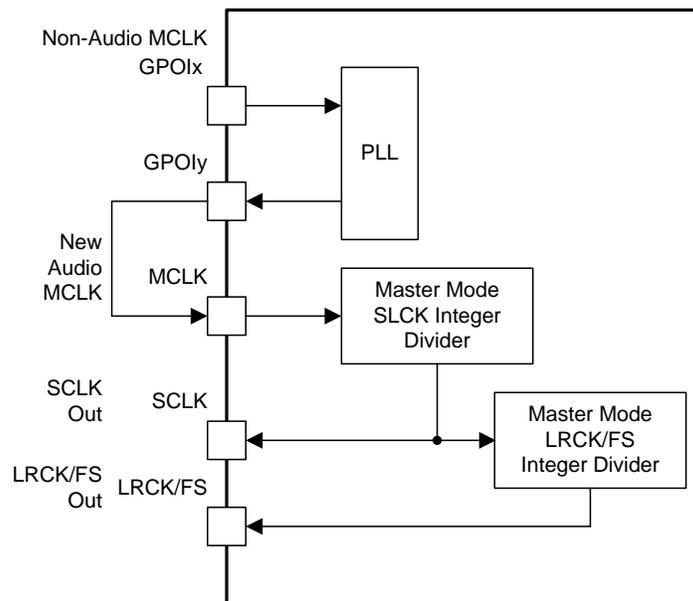
Figure 59. Generating Audio Clocks Using Non-Audio Clock Sources
