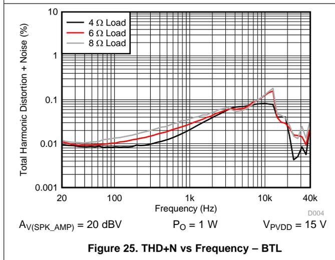
Figure 25. THD+N vs Frequency – BTL
