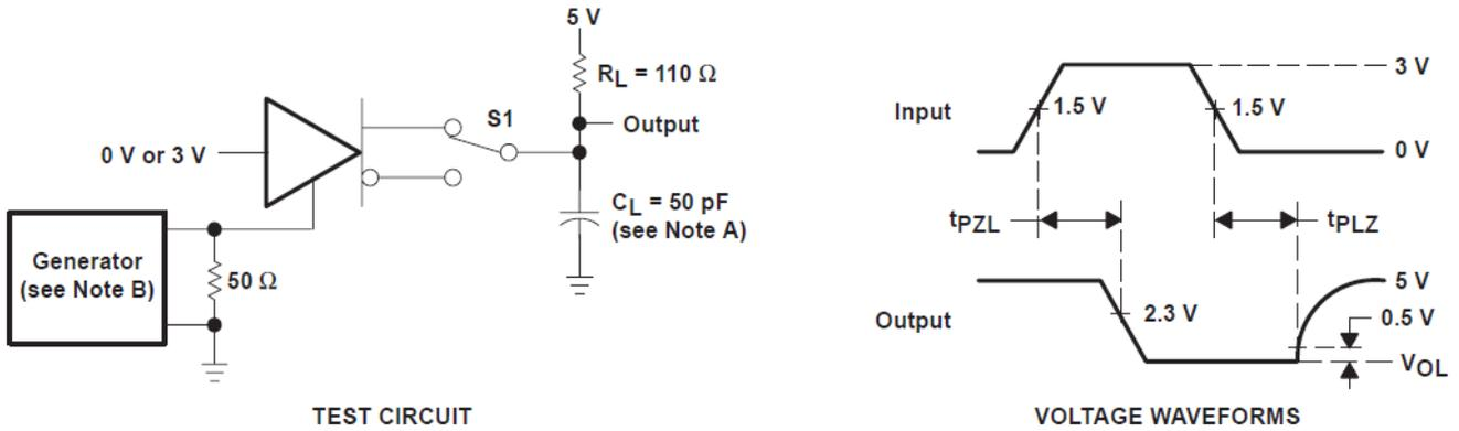
**图 6-5. Driver Test Circuit and Voltage Waveforms**
