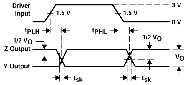
图 6-3. Driver Propagation Delay Times
