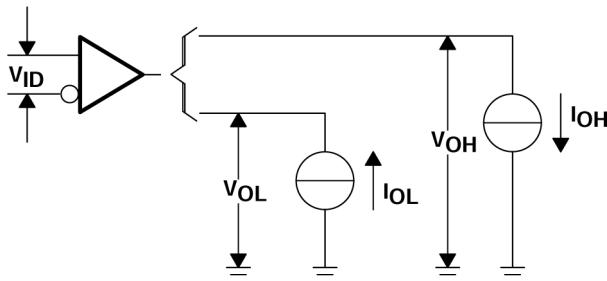
图 6-2. Receiver Test Circuit,  $V_{OH}$  and  $V_{OL}$
