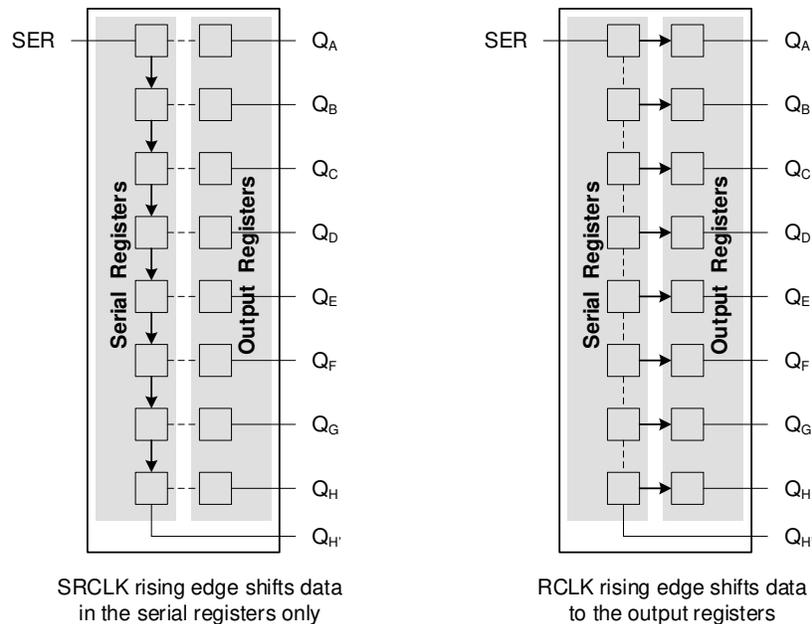
图 9-2. Simplified functional diagram showing clock operation
