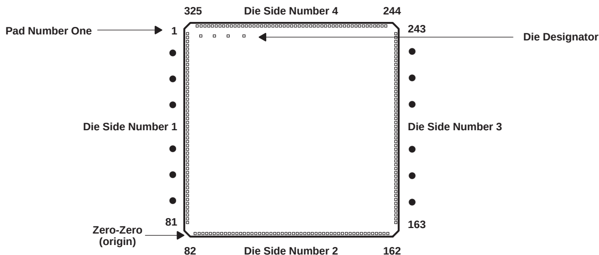
Figure 2. '320C40 Die Numbering Format (See Table 1)
