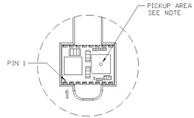
NOTE: THE INDUCTOR IS USED TO PICK AND PLACE THE MODULE. IT'S LOCATION MAY VARY FROM PACKAGE STYLE. SEE PRODUCT TABLE
