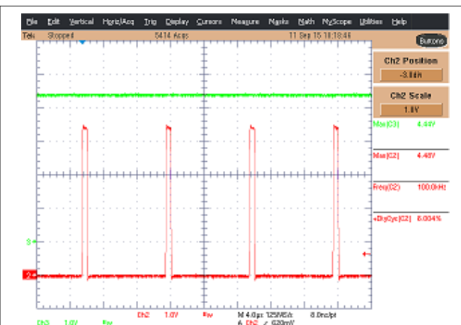
图 8-9. Supply Voltage 5 V Peak Signal 4.5 V
