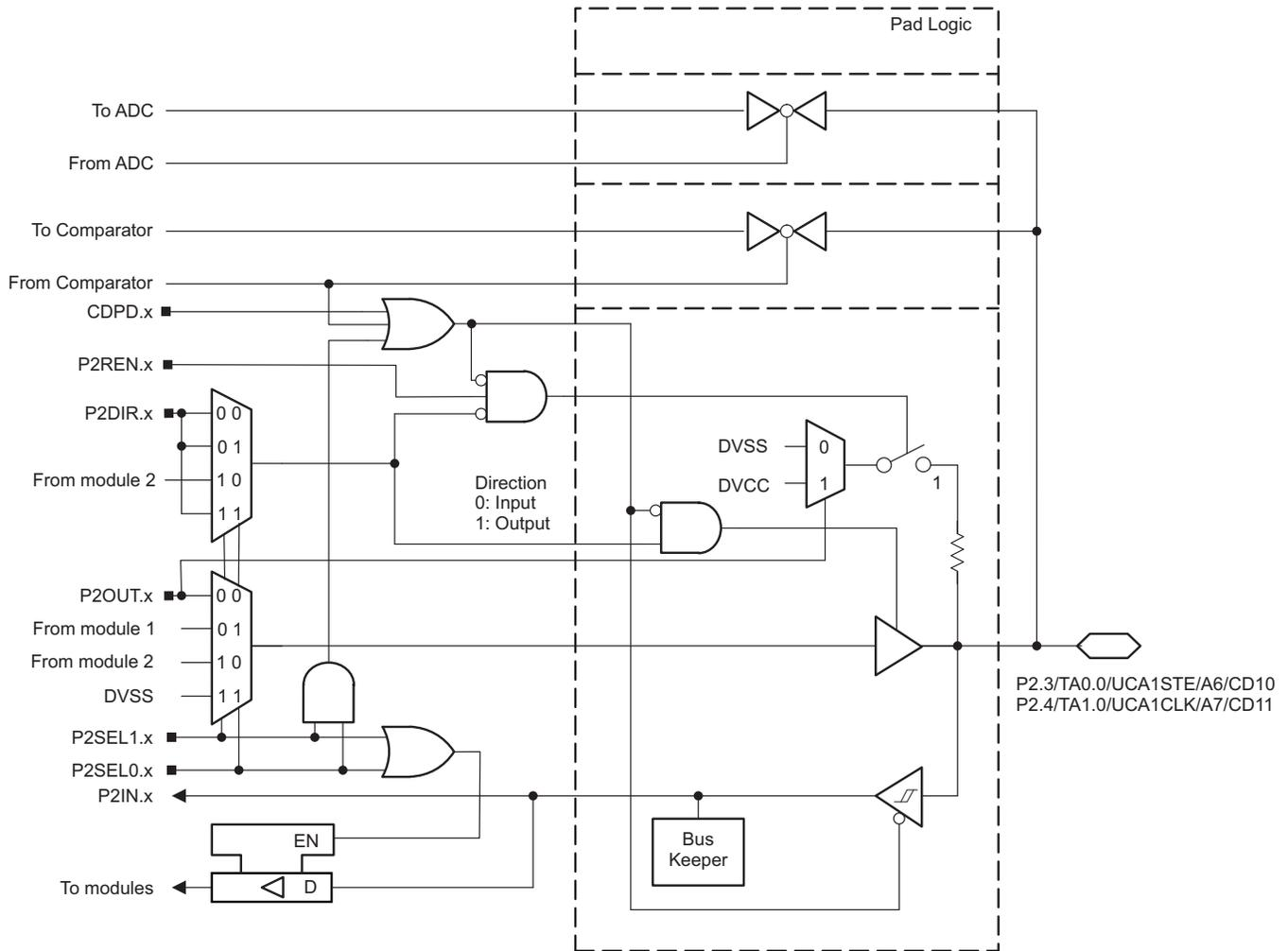
图 6-13. Port P2 (P2.3 and P2.4) Diagram
