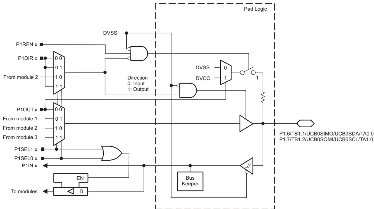
图 6-11. Port P1 (P1.6 and P1.7) Diagram
