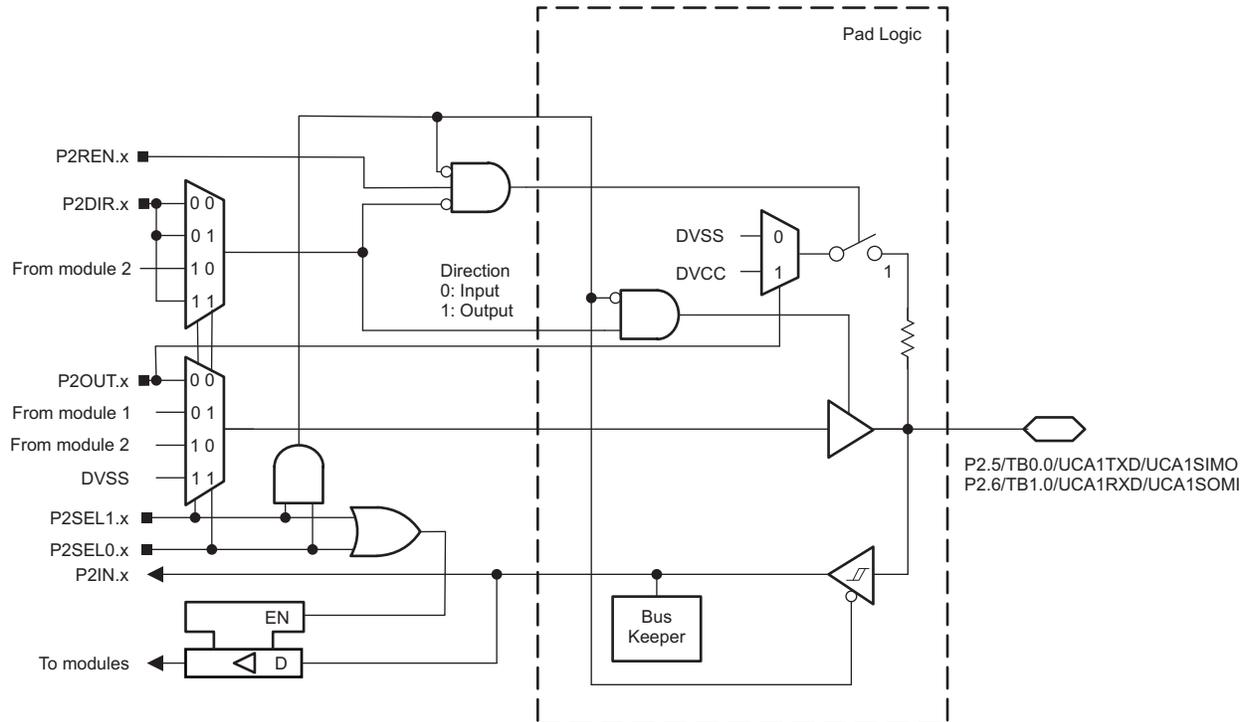
图 6-14. Port P2 (P2.5 and P2.6) Diagram
