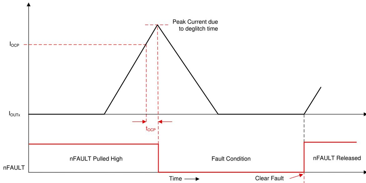
**图 7-51. Overcurrent Protection - Latched Shutdown Mode**
