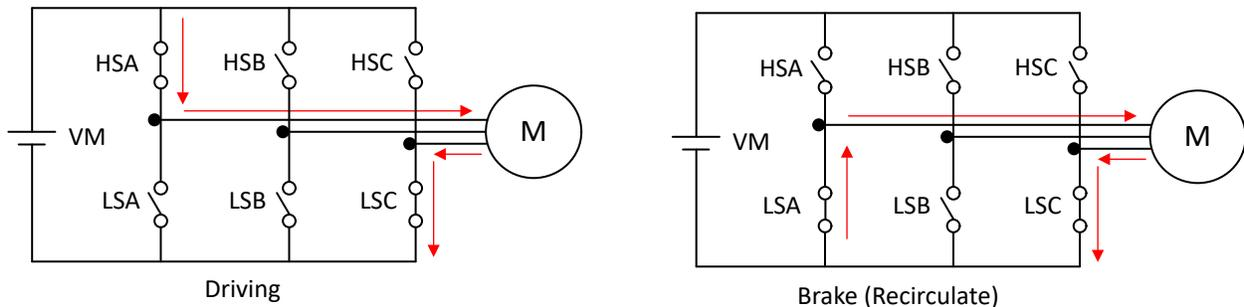
图 7-24. IPD Release Mode - Brake (0b)
