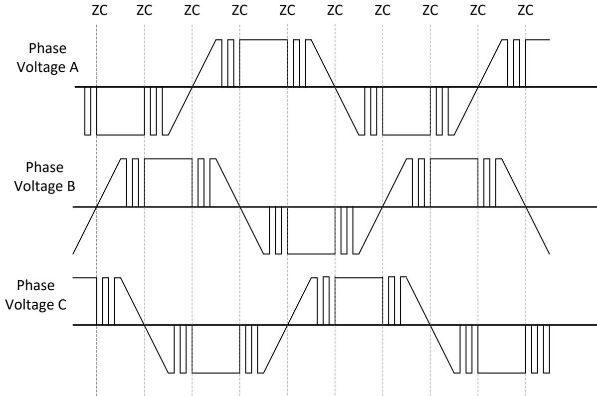
图 7-30. 120° commutation in Mixed Modulation Mode
