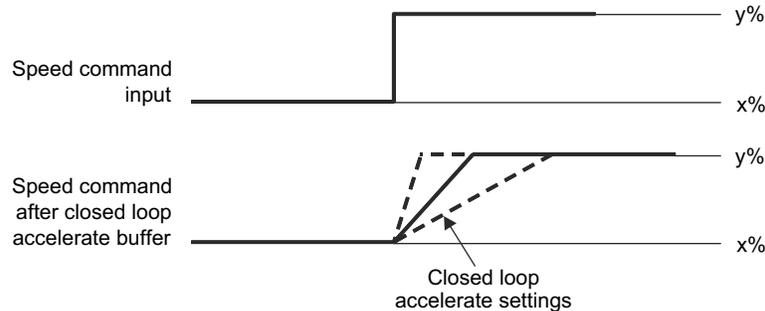
图 7-33. Closed loop accelerate
