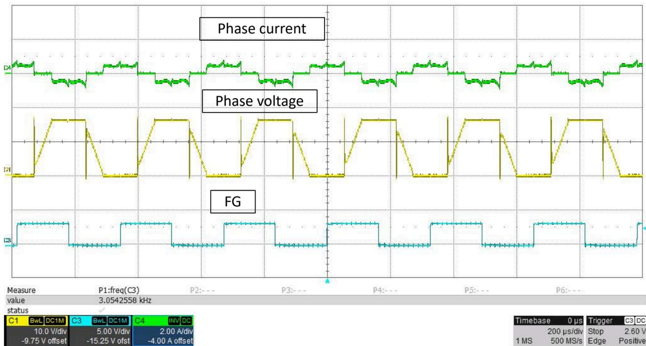
**图 8-7. Phase current, Phase voltage and FG at Maximum speed**
