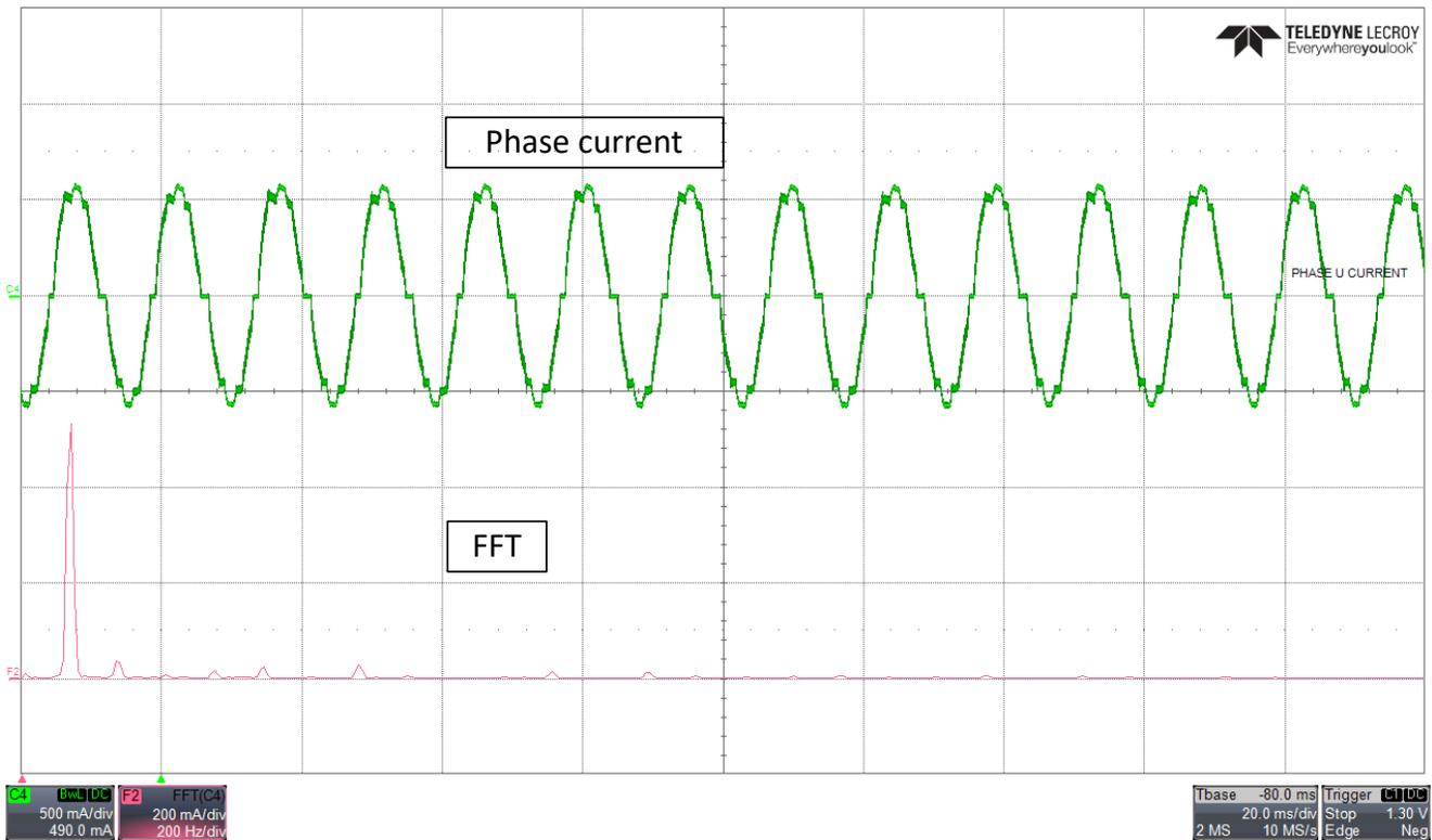
**图 8-4. Phase current and FFT - 150°commutation**
