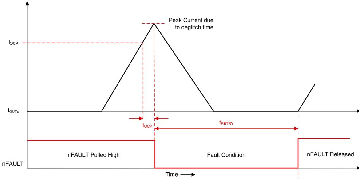
图 7-52. Overcurrent Protection - Automatic Retry Mode
