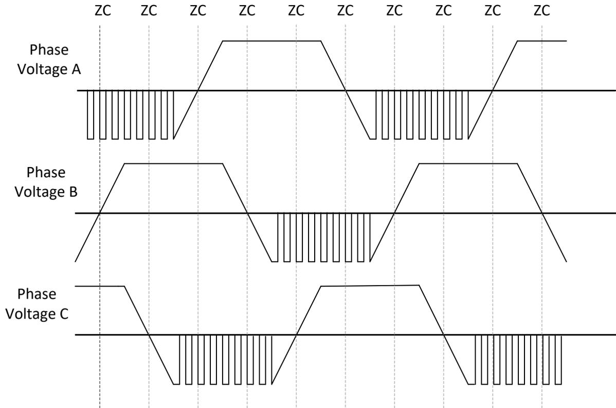
**图 7-29. 120 ° commutation in Low Side Modulation Mode**
