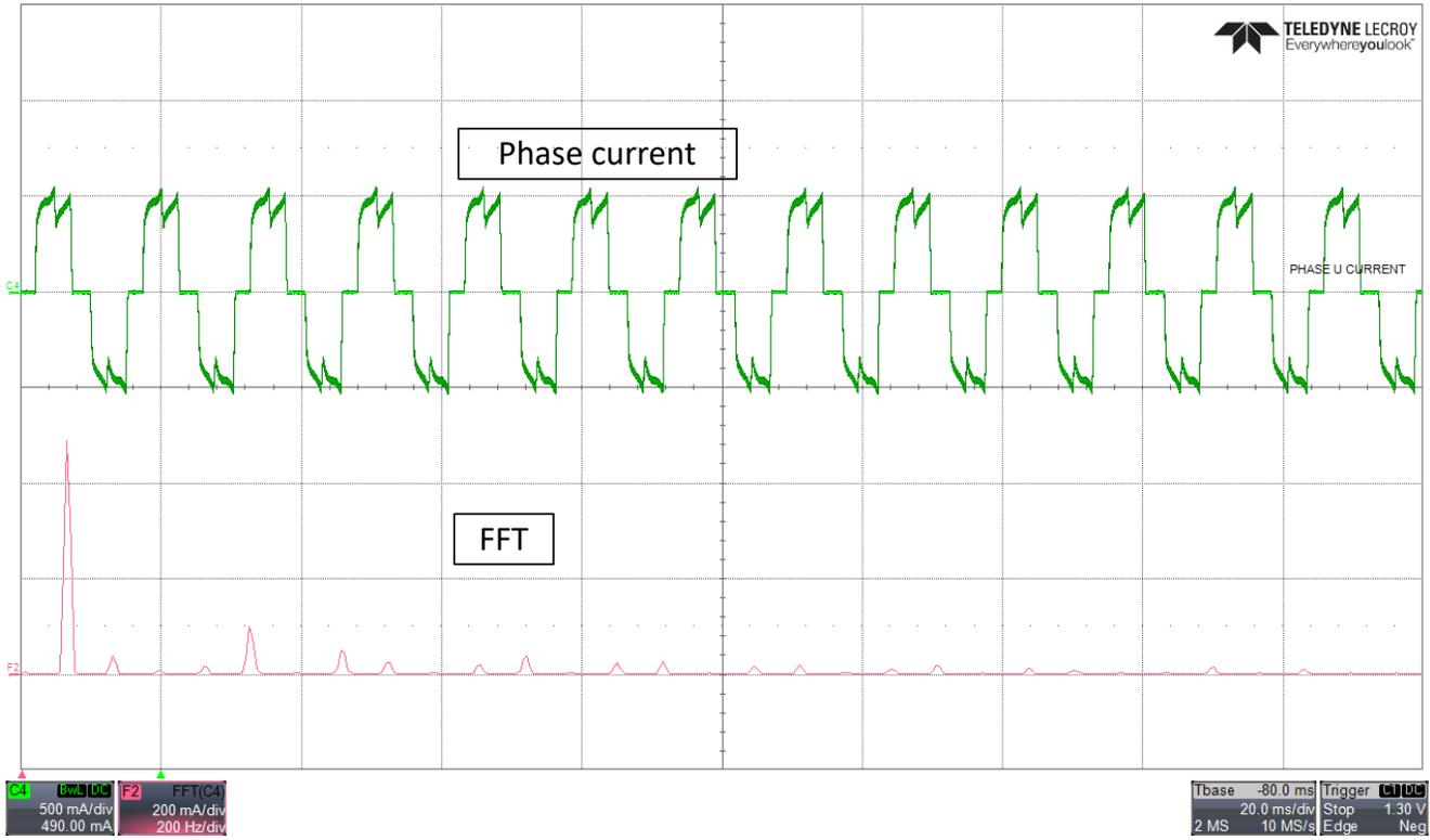
**图 8-3. Phase current and FFT - 120 °commutation**
