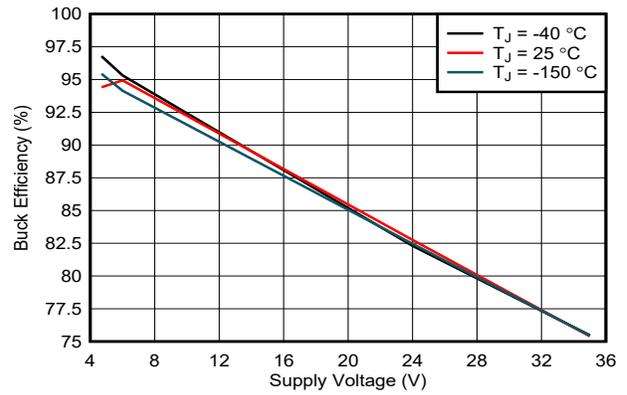
图 6-2. Buck regulator efficiency over supply voltage
