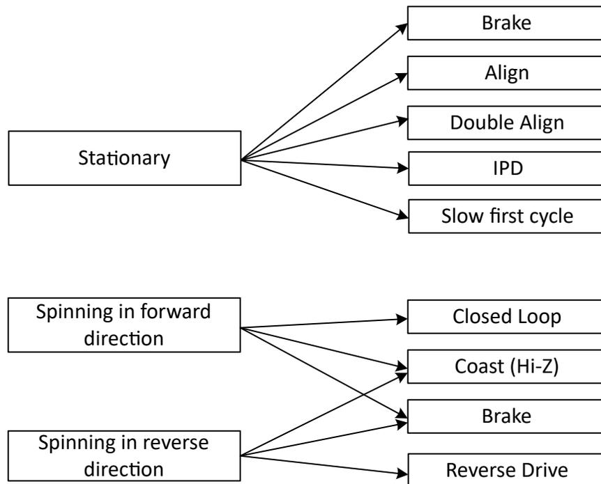
图 7-19. Starting the motor under different initial conditions
