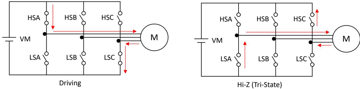
图 7-25. IPD Release Mode - Tristate (1b)
