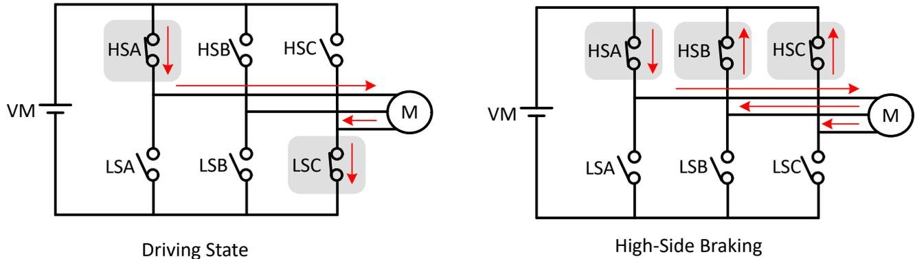
图 7-46. High-Side Braking
