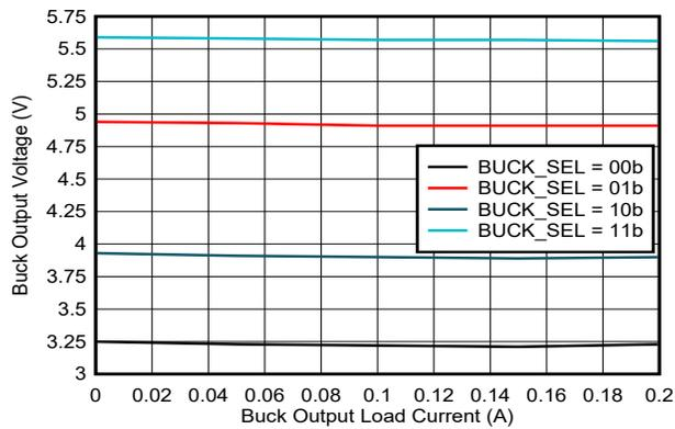
图 6-3. Buck regulator output voltage over load current
