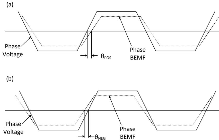
图 7-32. Positive and Negative Lead Angle Definition
