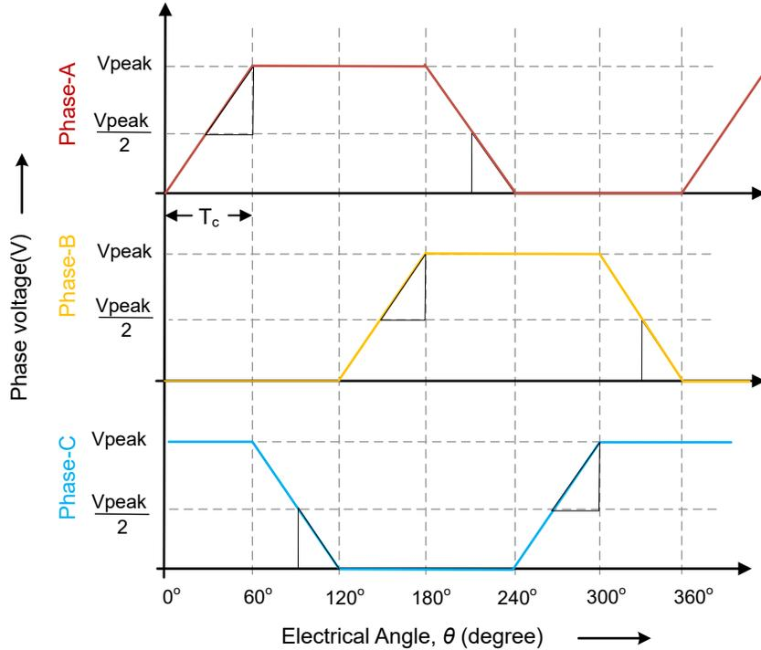
图 7-37. Back-EMF integration using floating phase voltage
