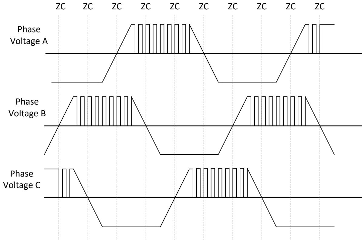
图 7-28. 120° commutation in High Side Modulation Mode
