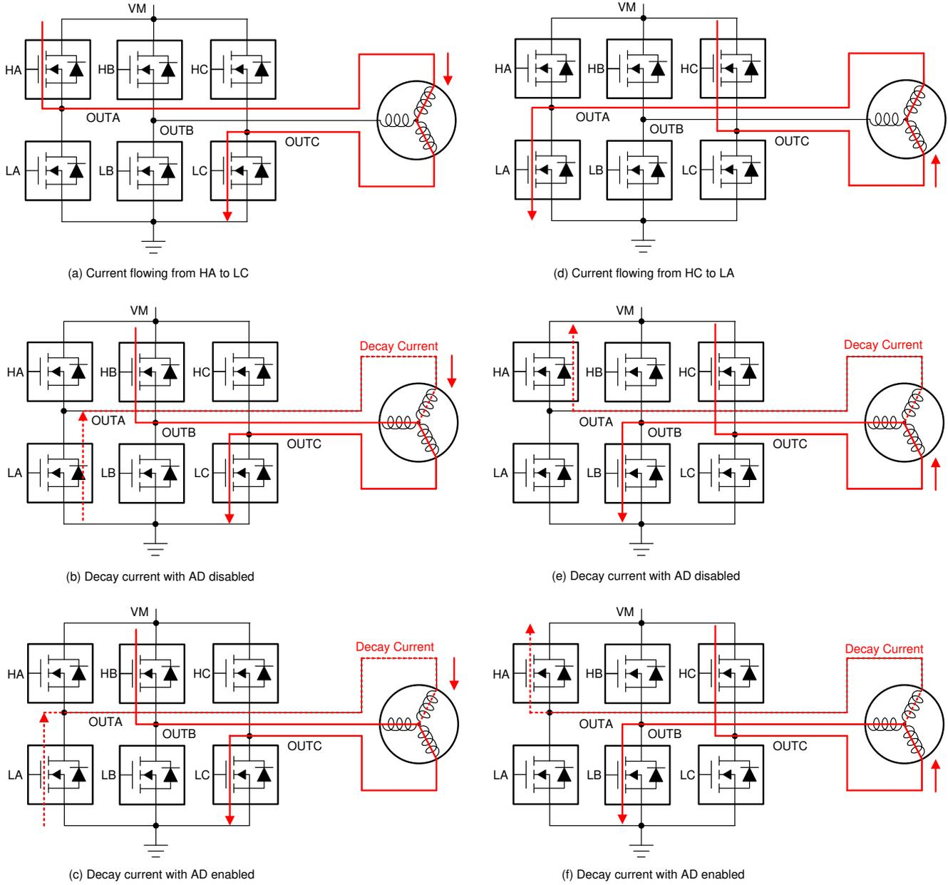
**图 7-40. Active Demagnetization in BLDC Motor Commutation**
