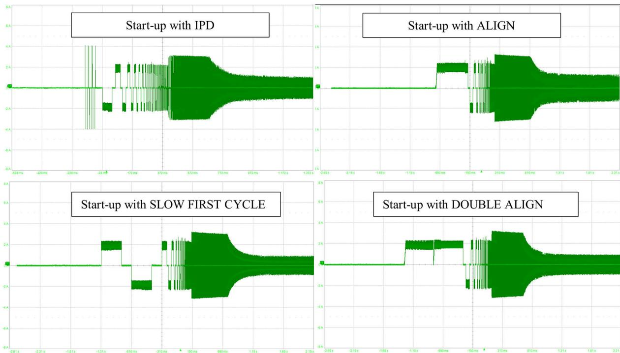
图 8-2. Motor phase current waveforms of all startup methods
