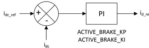
图 7-42. Active Braking Current Control Loop for  $i_{d\_ref}$
