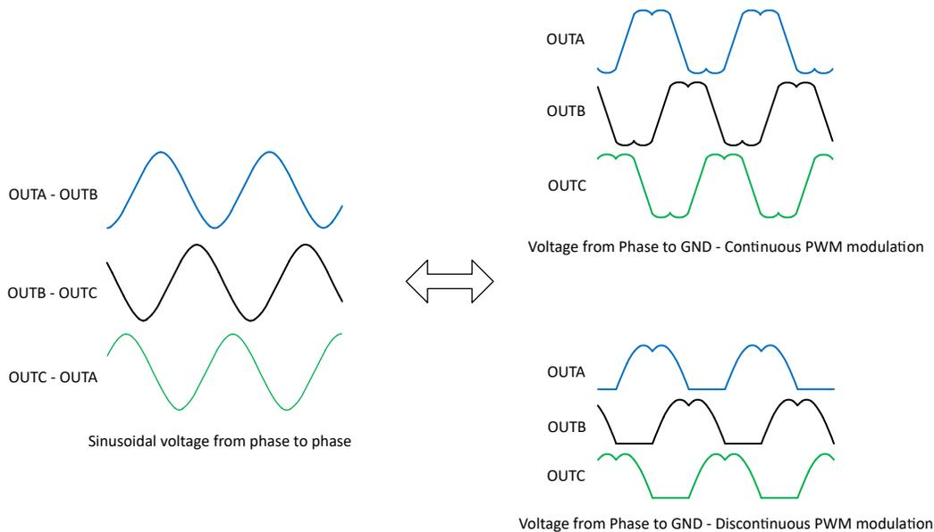
图 7-43. Continuous and Discontinuous PWM Modulation Phase Voltages
