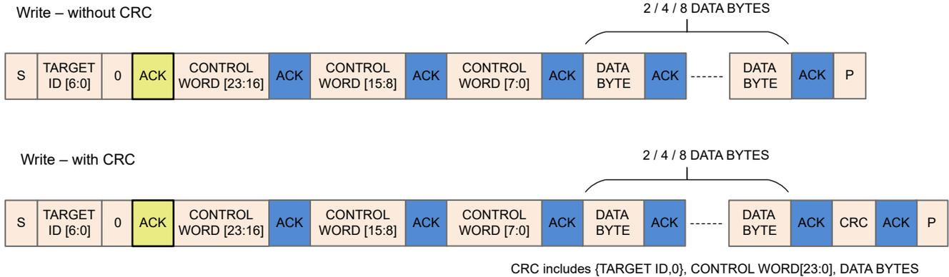
**图 7-57. I<sup>2</sup>C Write Transaction Sequence**
