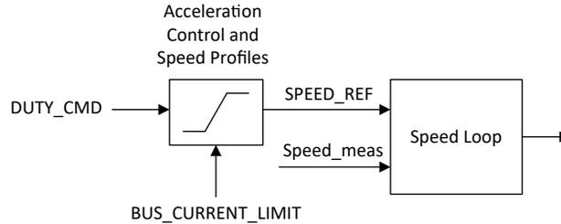
图 7-51. DC Bus Current Limit Functional Block Diagram
