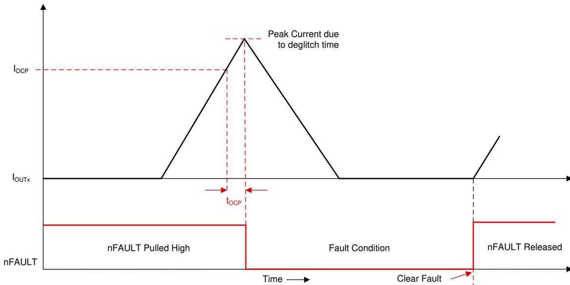
图 7-54. Overcurrent Protection - Latched Shutdown Mode
