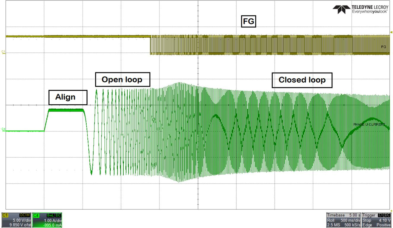
图 8-3. Motor Startup - FG and Phase current
