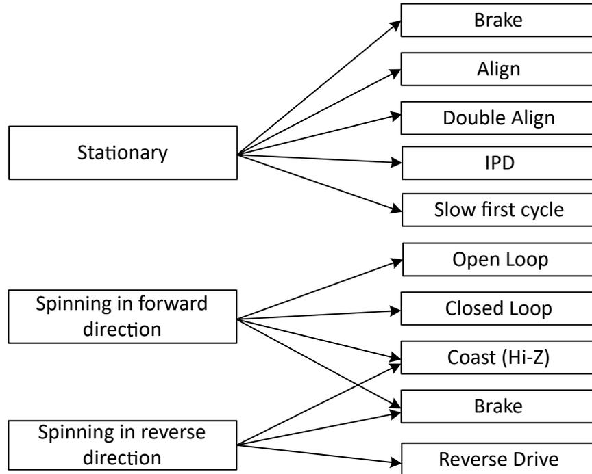
图 7-22. Starting the motor under different initial conditions
