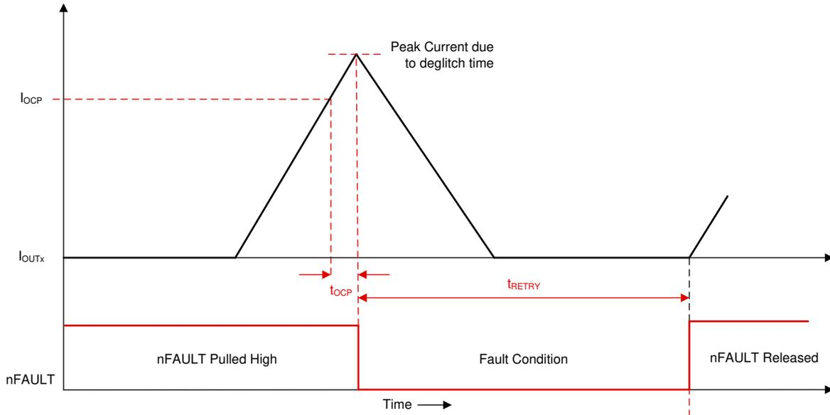
图 7-55. Overcurrent Protection - Automatic Retry Mode
