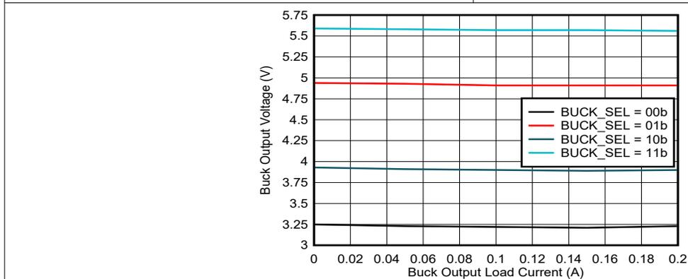
图 6-3. Buck regulator output voltage over load current
