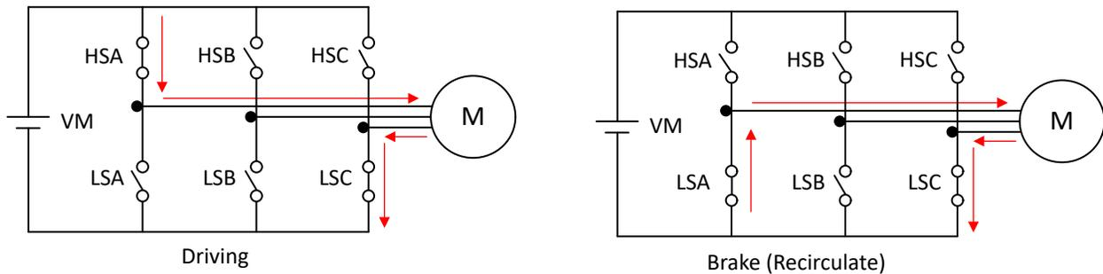
图 7-27. IPD Release Mode - Brake (0b)
