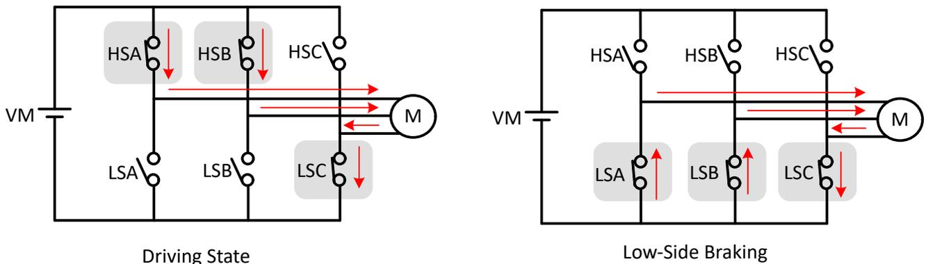
图 7-47. Low-Side Braking
