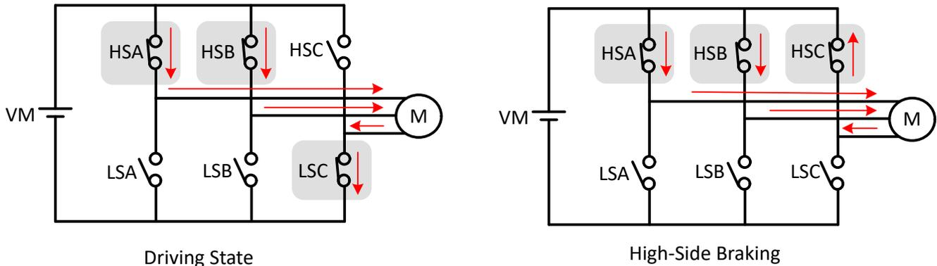
图 7-48. High-Side Braking
