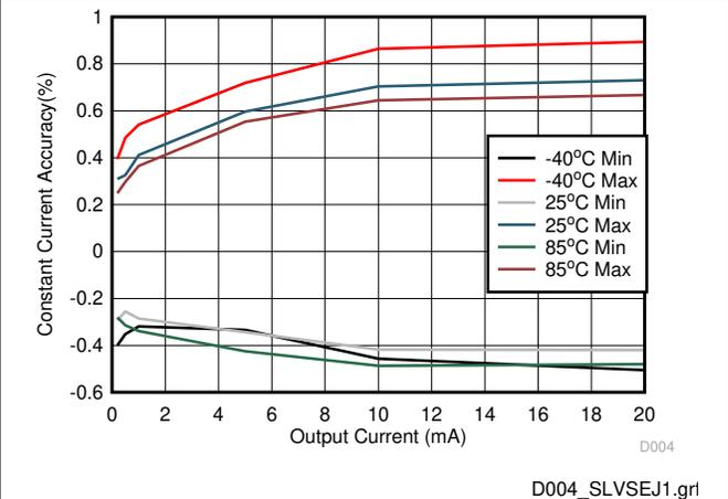
图 7-5. Channel to Channel Accuracy vs Output Current
