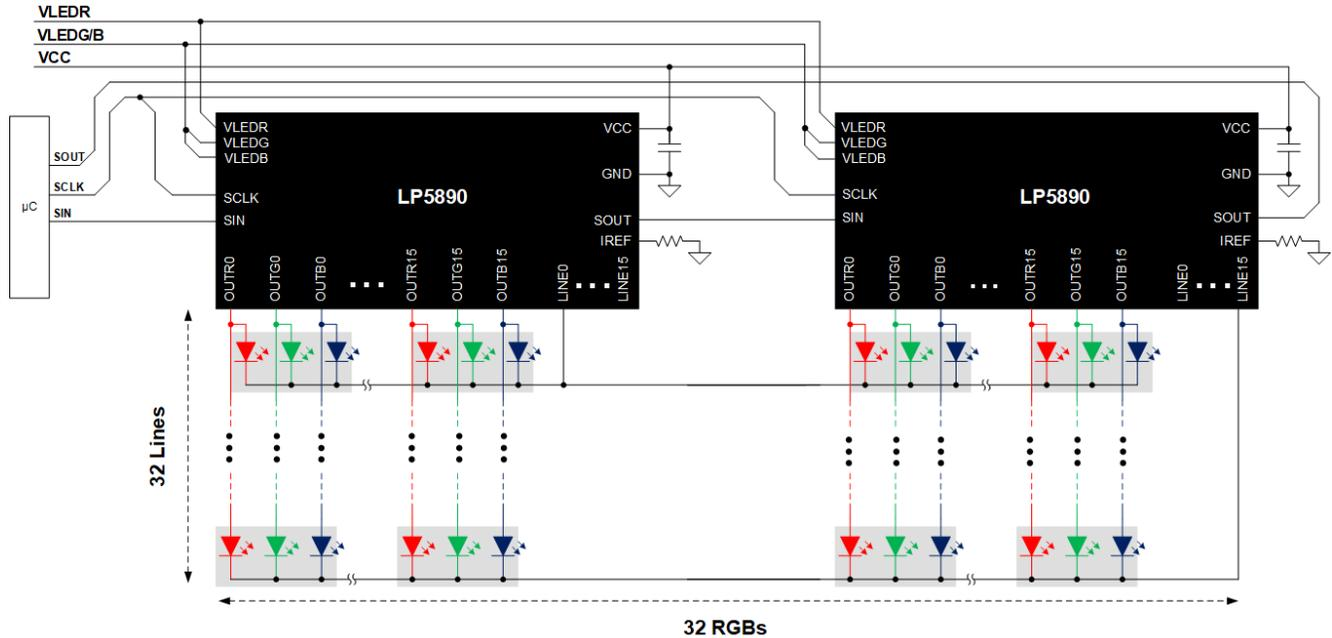
图 9-1. LP5890 with Dual Devices Stackable Connection
