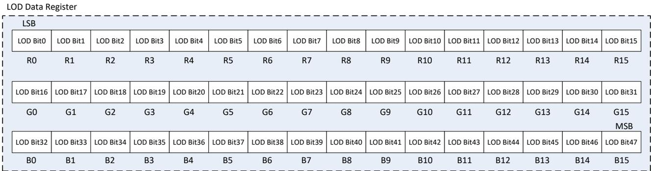
图 8-6. Bit Arrangement in LOD Data Register
