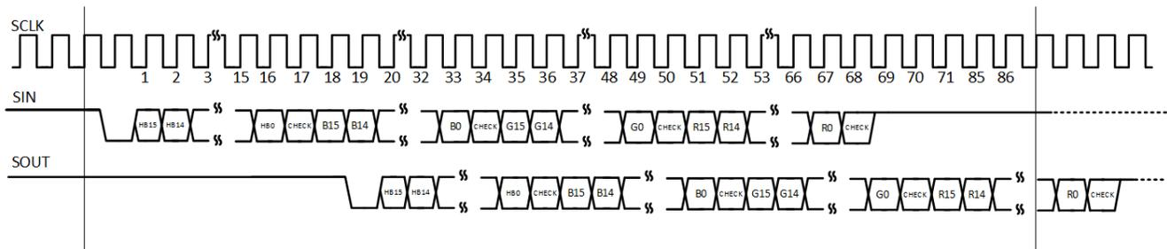
图 8-18. Data Write Command With Broadcast (Timing Diagram)
