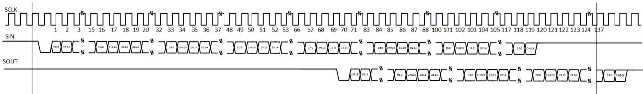
图 8-20. Data Write Command with Non-Broadcast (Timing Diagram)
