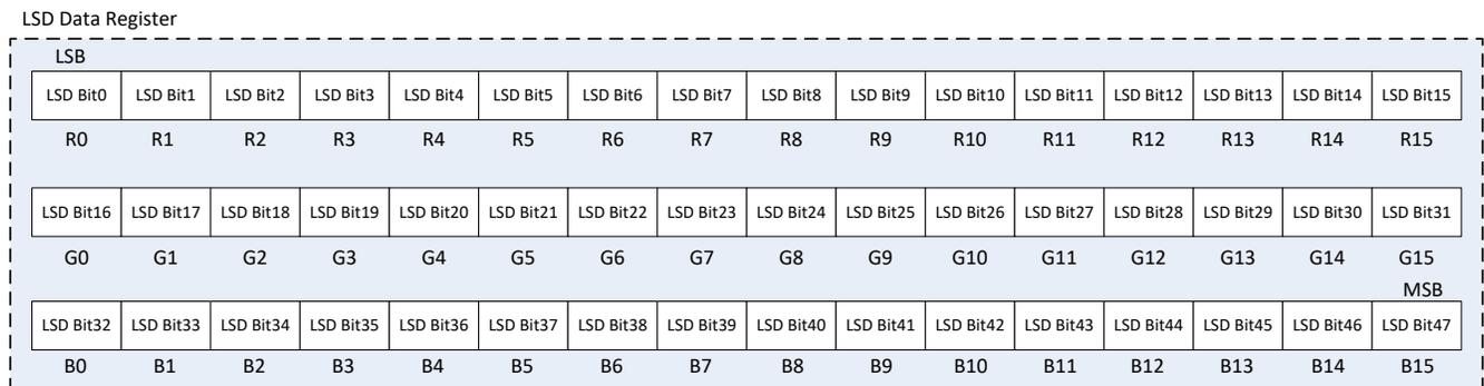
图 8-10. Bit Arrangement in the LSD Data Register
