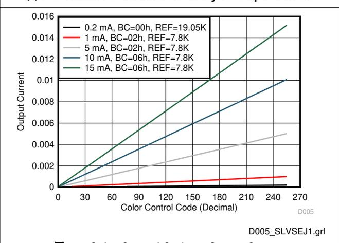
图 7-7. Color Control Code vs Output Current
