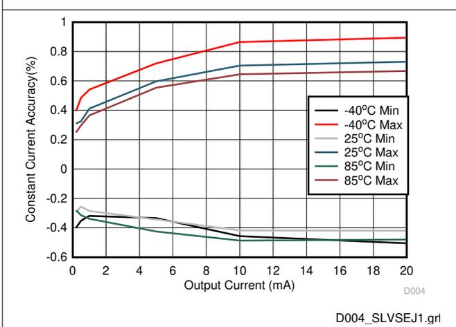
图 7-6. Channel to Channel Accuracy vs Output Current
