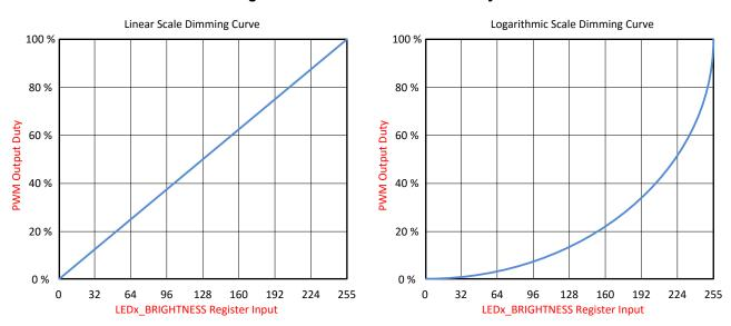
图 7-3. Logarithmic vs Linear Dimming Curve
