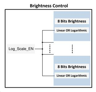
图 7-2. Logarithmic- or Linear-Scale Intensity Control
