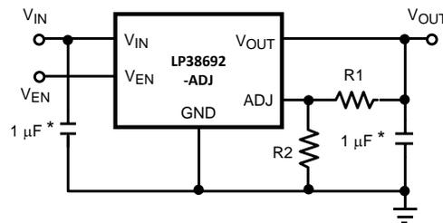
$$V_{\text{输出}} = V_{\text{ADJ}} \times (1 + R1/R2)$$
