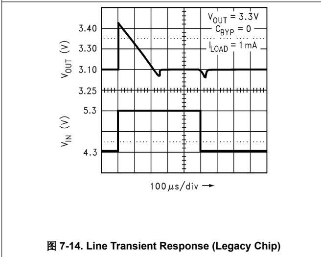
图 7-14. Line Transient Response (Legacy Chip)
