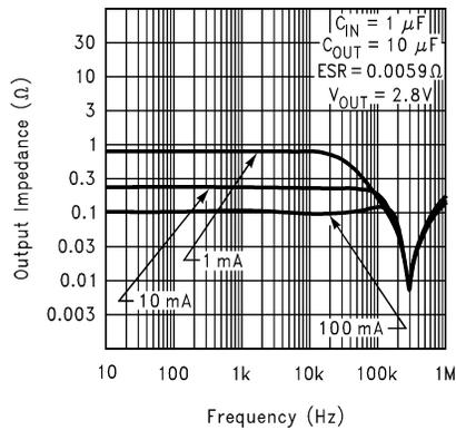
图 5-17. Output Impedance vs Frequency (Legacy Chip)
