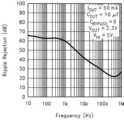
图 5-7. Ripple Rejection vs Frequency (Legacy Chip)
