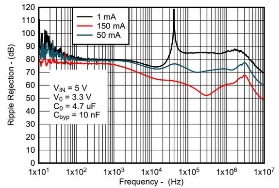
图 5-16. Ripple Rejection vs Frequency (New Chip)
