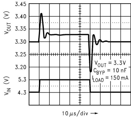
图 7-20. Line Transient Response (Legacy Chip)
