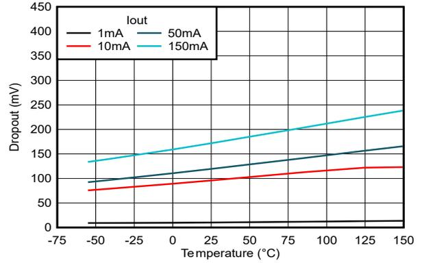
图 5-26. Dropout Voltage vs Temperature (New Chip)
