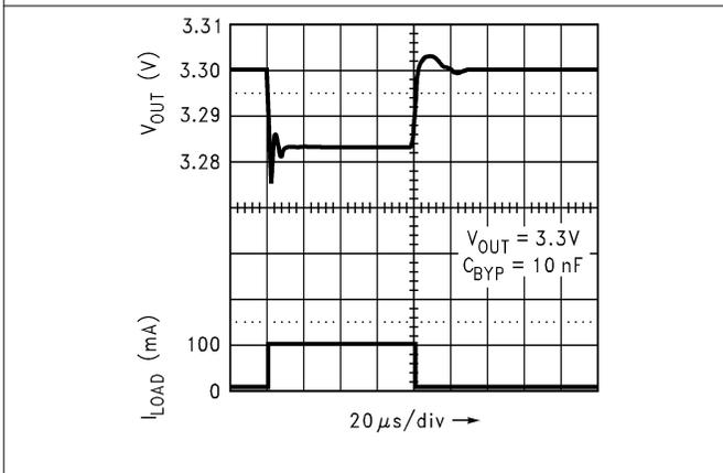
图 7-8. Load Transient Response (Legacy Chip)
