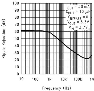
图 5-11. Ripple Rejection vs Frequency (Legacy Chip)
