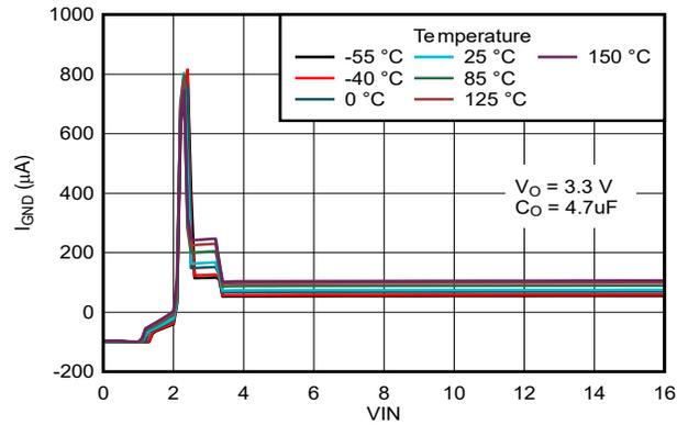
图 5-28. Input Current vs V\_IN (New Chip)
