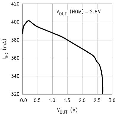
图 5-3. Short-Circuit Current vs Output Voltage (Legacy Chip)
