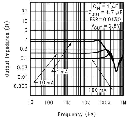
图 5-18. Output Impedance vs Frequency (Legacy Chip)
