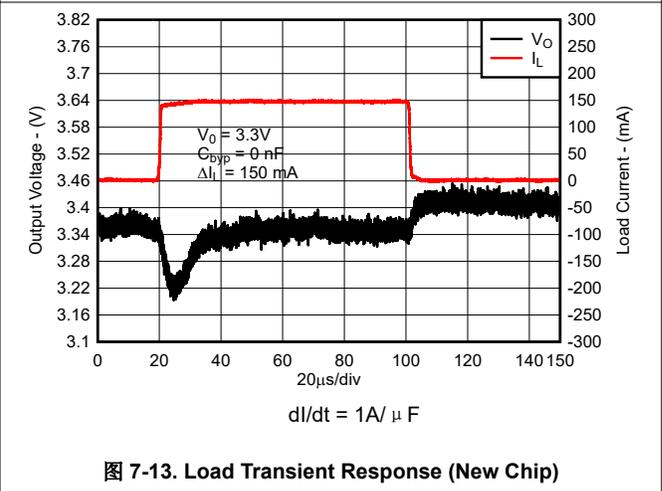
图 7-13. Load Transient Response (New Chip)
