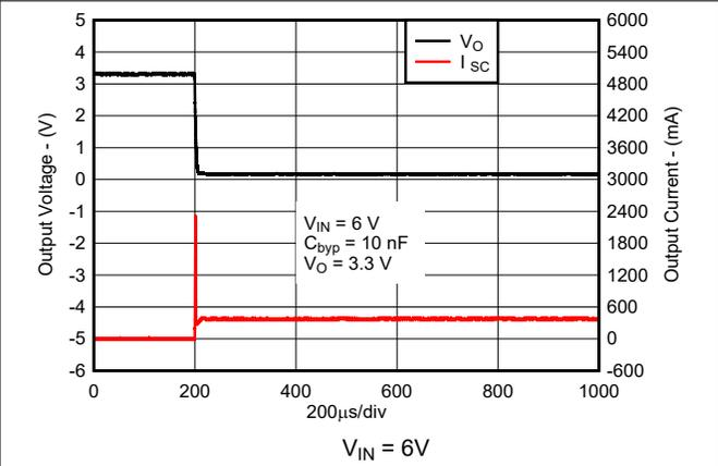
图 7-5. Short-Circuit Current (New Chip) at  $V_{IN} = 6\text{V}$
