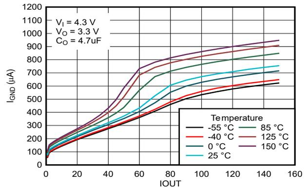
图 5-24. Ground Pin Current vs Load Current (New Chip)
