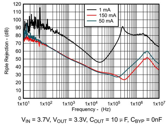
图 5-14. Ripple Rejection vs Frequency (New Chip)
