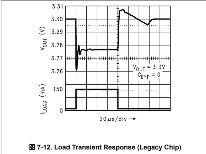
图 7-12. Load Transient Response (Legacy Chip)
