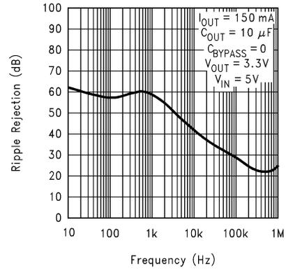
图 5-8. Ripple Rejection vs Frequency (Legacy Chip)
