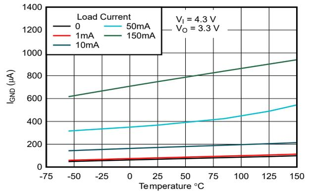
图 5-30. GND Pin Current vs Temperature (New Chip)
