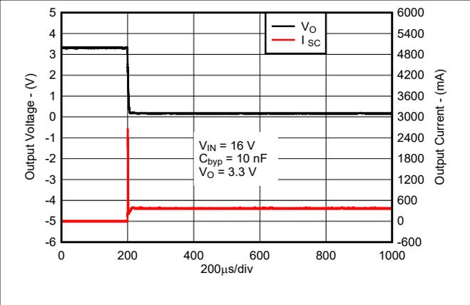
图 7-7. Short-Circuit Current (New Chip) at  $V_{IN} = 16\text{V}$
