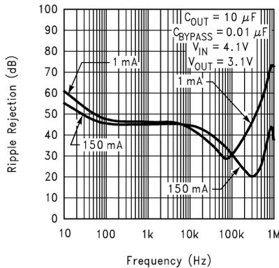
图 5-5. Ripple Rejection vs Frequency (Legacy Chip)
