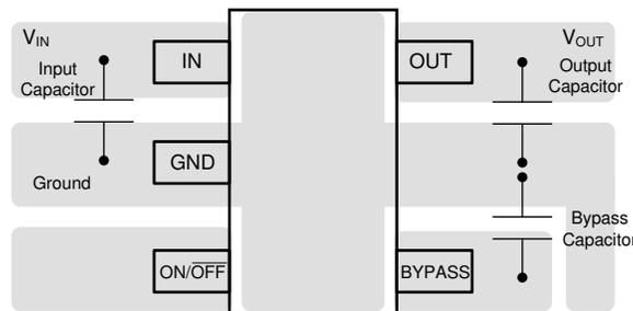
图 7-30. LP2985 SOT-23 Package Typical Layout
