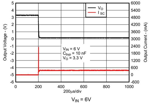
图 7-5. Short-Circuit Current (New Chip) at  $V_{IN} = 6\text{V}$
