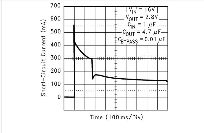
图 7-6. Short-Circuit Current (Legacy Chip) at  $V_{IN} = 16\text{V}$
