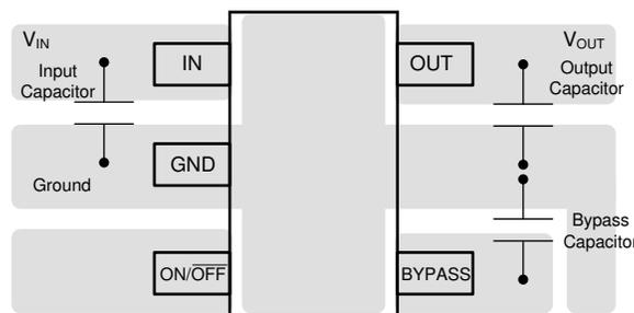
图 7-30. LP2985 SOT-23 Package Typical Layout
