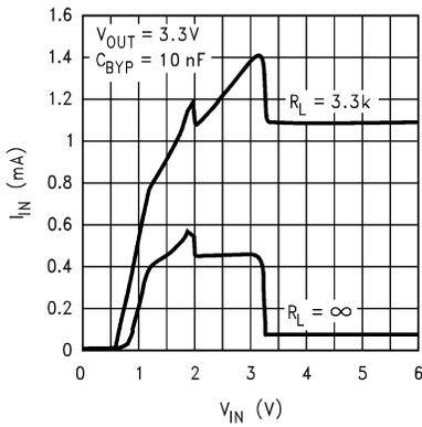
图 5-27. Input Current vs V\_IN (Legacy Chip)
