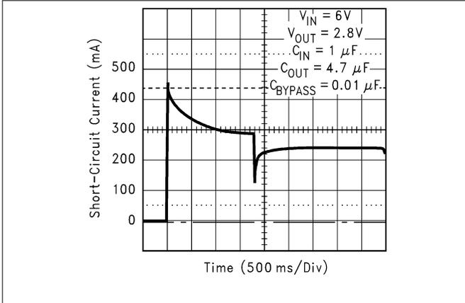
图 7-4. Short-Circuit Current (Legacy Chip) at  $V_{IN} = 6\text{V}$
