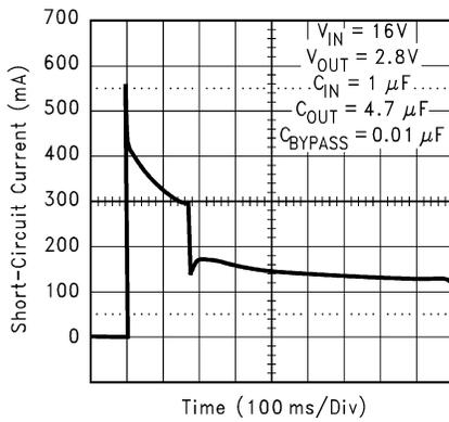
图 7-6. Short-Circuit Current (Legacy Chip) at  $V_{IN} = 16\text{V}$
