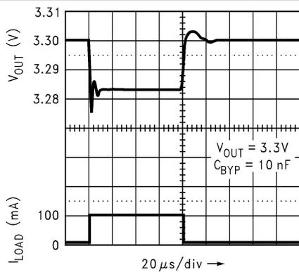
图 7-8. Load Transient Response (Legacy Chip)
