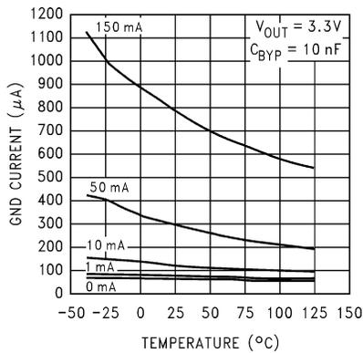
图 5-29. GND Pin Current vs Temperature (Legacy Chip)
