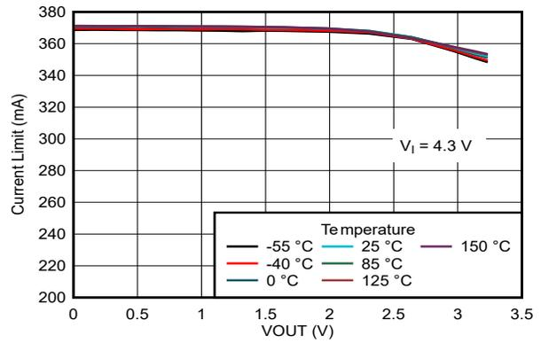
图 5-4. Short-Circuit Current vs Output Voltage (New Chip)
