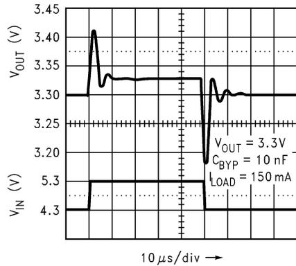
图 7-20. Line Transient Response (Legacy Chip)
