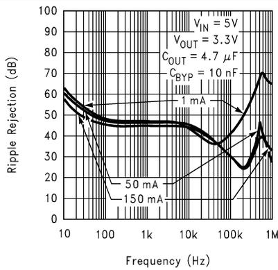
图 5-15. Ripple Rejection vs Frequency (Legacy Chip)
