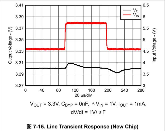
图 7-15. Line Transient Response (New Chip)
