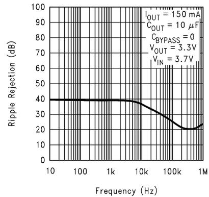
图 5-12. Ripple Rejection vs Frequency (Legacy Chip)
