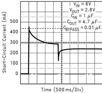
图 7-4. Short-Circuit Current (Legacy Chip) at  $V_{IN} = 6\text{V}$
