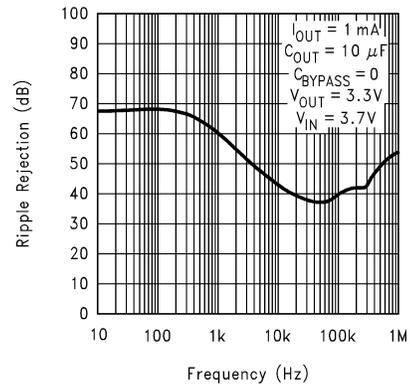
图 5-10. Ripple Rejection vs Frequency (Legacy Chip)
