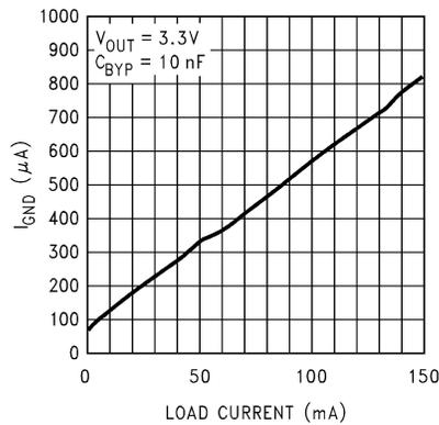
图 5-23. Ground Pin vs Load Current (Legacy Chip)
