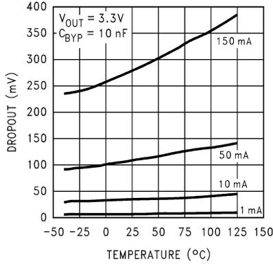
图 5-25. Dropout Voltage vs Temperature (Legacy Chip)
