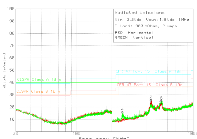
Figure 35. Radiated Emissions 3.3-V Input, 1.8-V Output, 2-A Load (EN55022 Class B)
