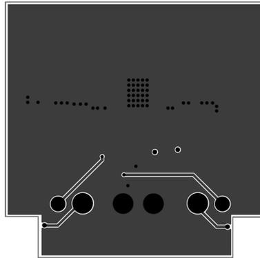
**Figure 33. Internal Layer 2 (Ground and Signal Traces)**
