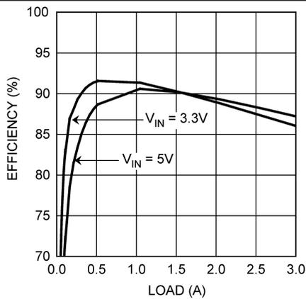
$V_{OUT} = 1.2\text{ V}$
