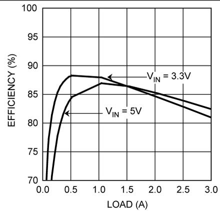
$V_{OUT} = 0.8\text{ V}$
