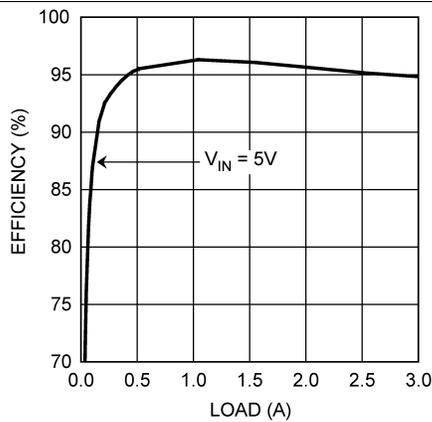
$V_{OUT} = 3.3\text{ V}$
